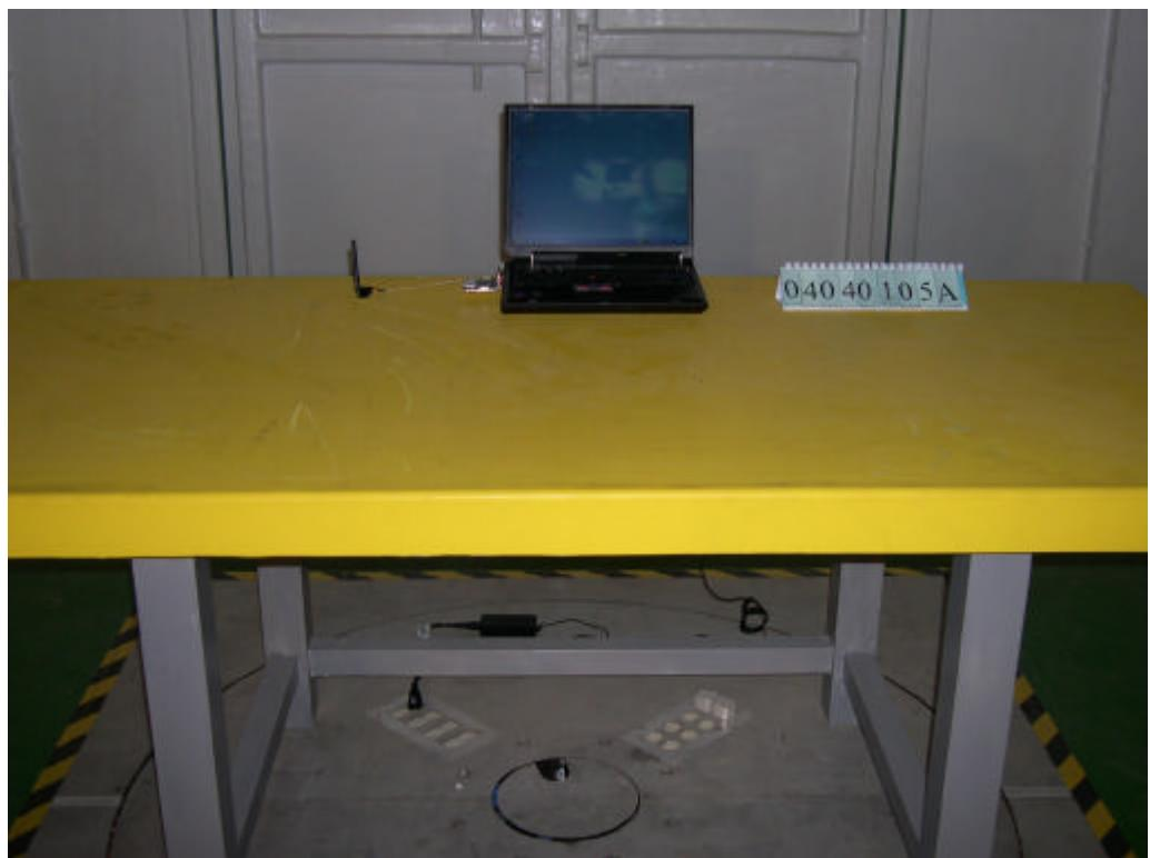
Radiated test. (back side)
