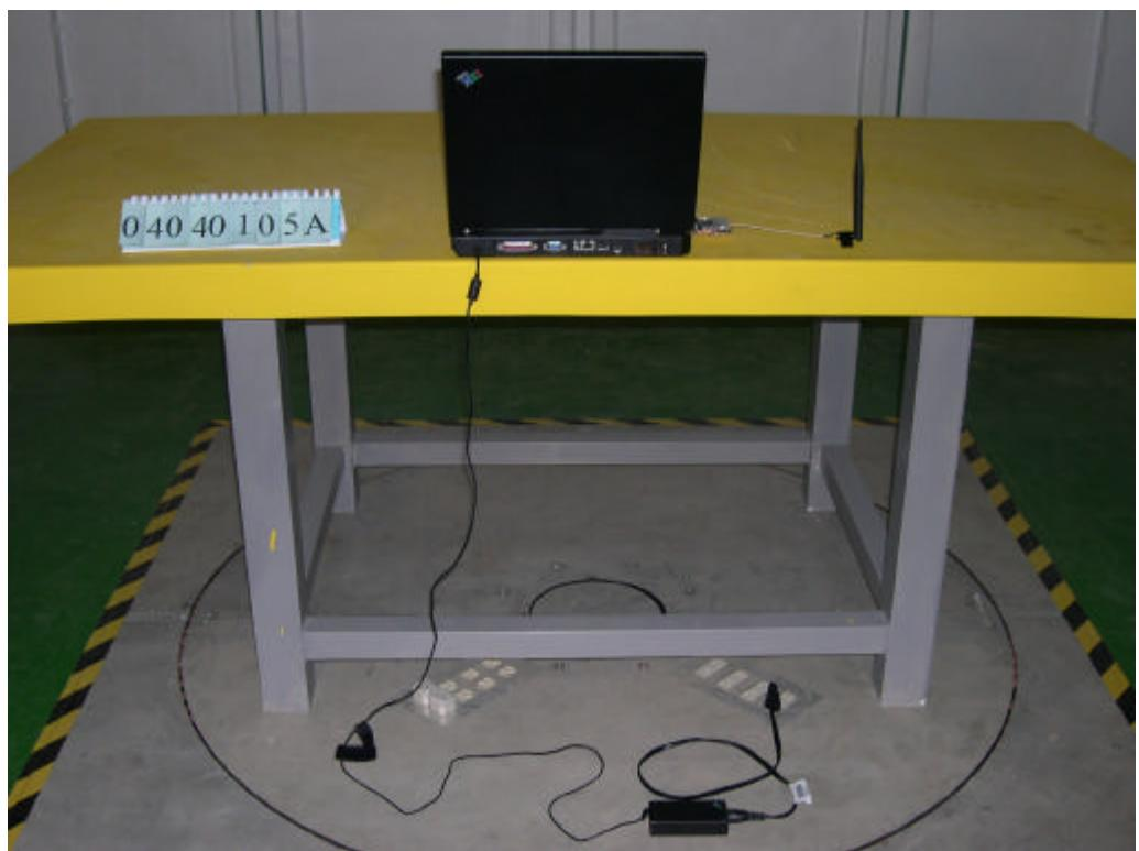
Radiated test. (front side)
