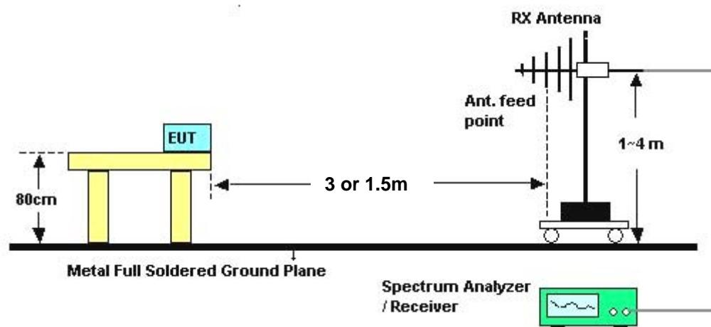
Above 10 GHz shall be extrapolated to the specified distance using an extrapolation factor of 20 dB/decade from 3m to 1.5m.
