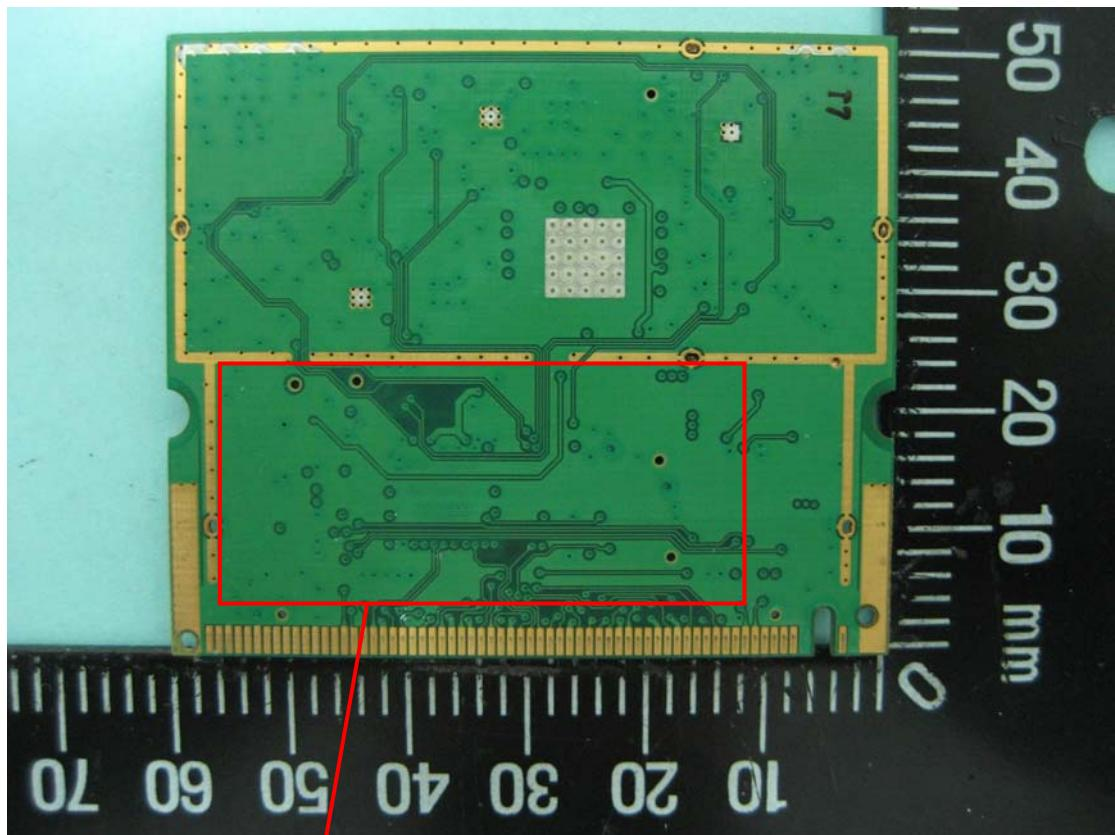
**802.11n compliant 2.4GHz Mini-PCI Module**
