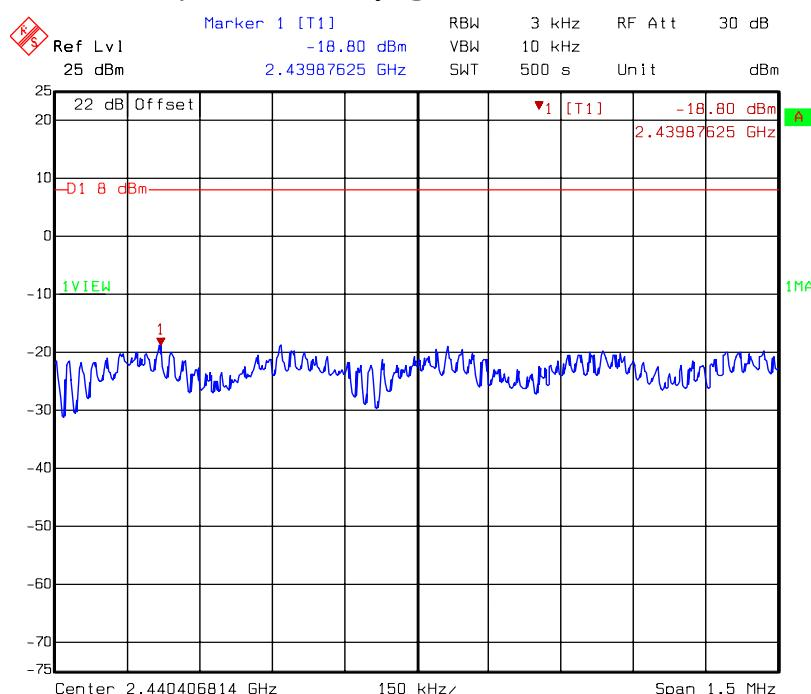
**DAC0 :Power Spectral Density @ 802.11n HT20 mode channel 11**
