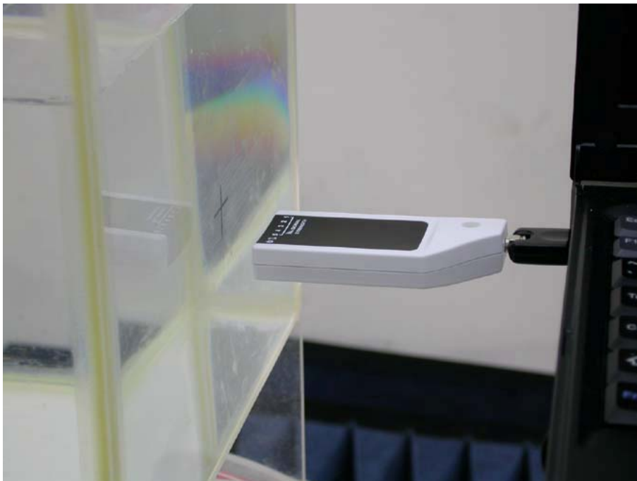
Figure 11: EUT perpendicular to phantom, 15 mm separation (with EUT lie down) - Zoom In
