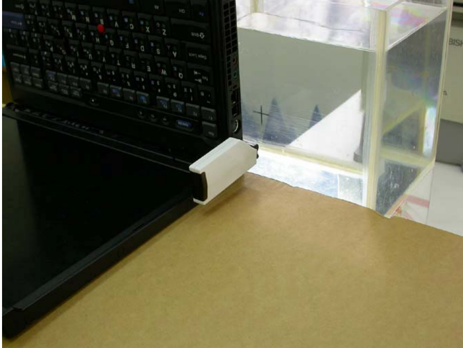
Figure 4: Bottom side of Laptop facing phantom touching with EUT stand
