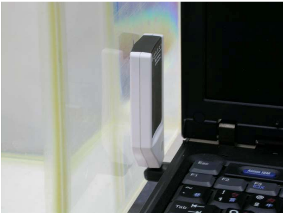
Figure 9: EUT perpendicular to phantom, 0 mm separation (with EUT stand) - Zoom In
