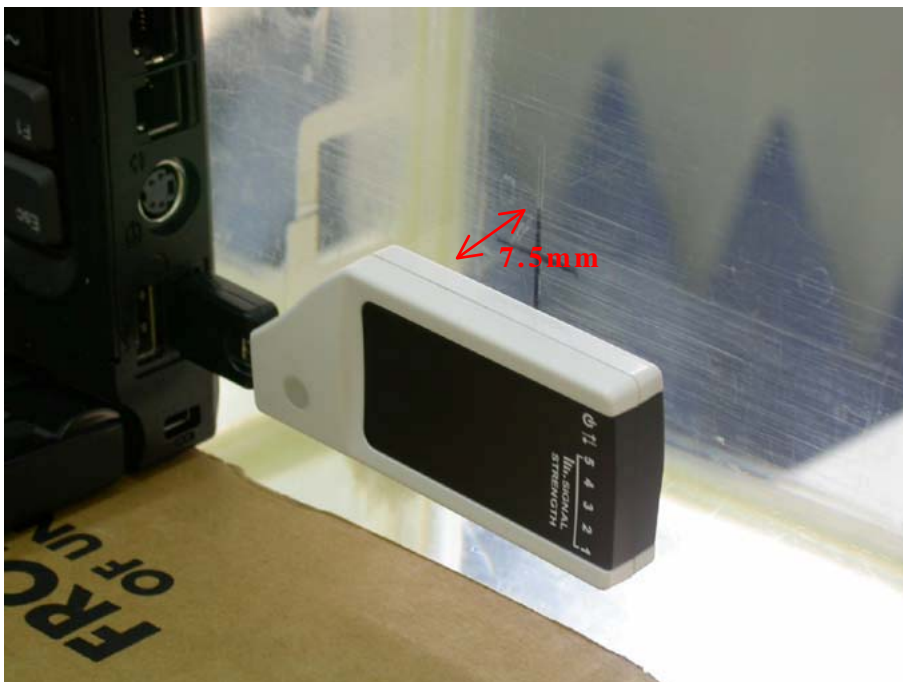
Figure 3: Bottom side of Laptop facing phantom touching with EUT lie down - Zoom In
