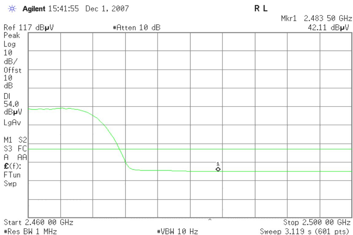
**Detector mode: Peak****Polarity: Horizontal**
