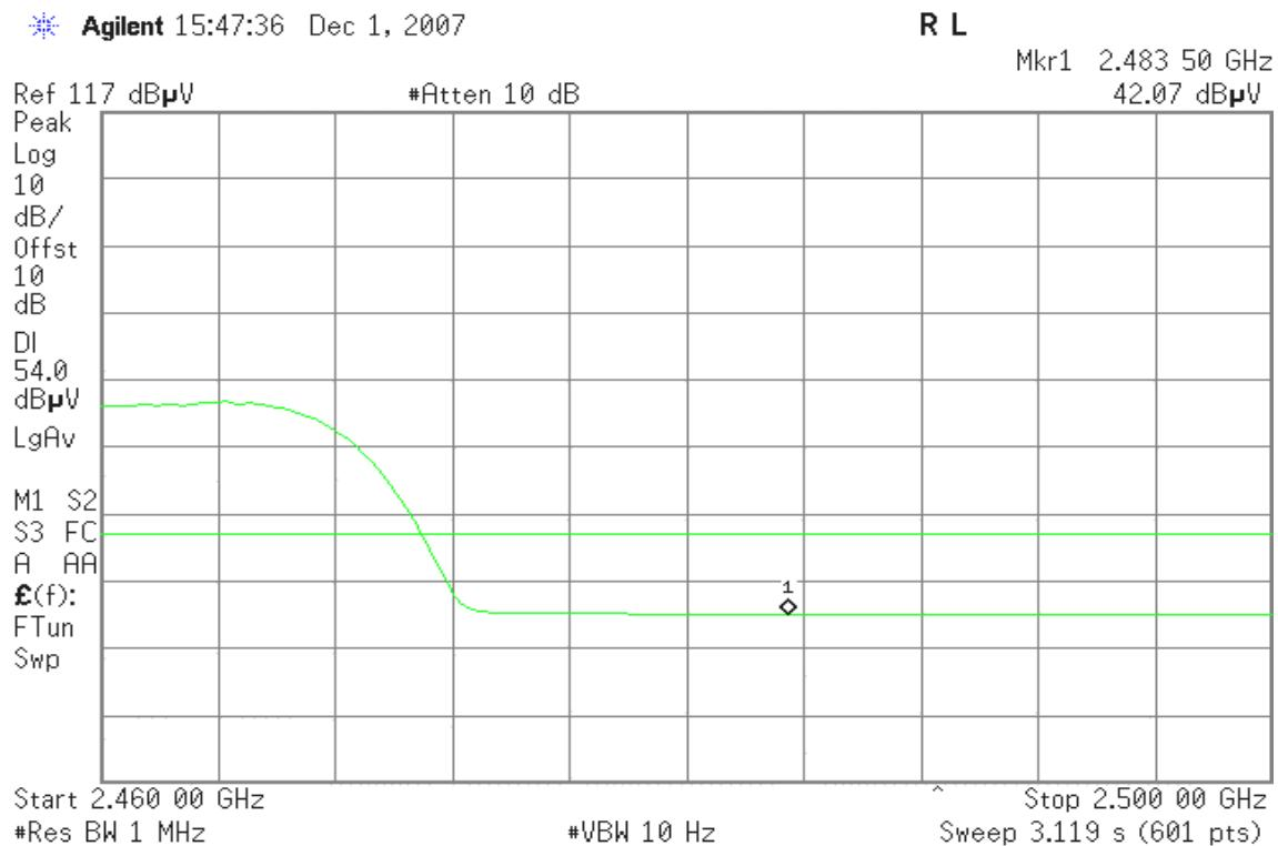
**Band Edges (IEEE 802.11g / CH Low)****Detector mode: Peak****Polarity: Vertical**
