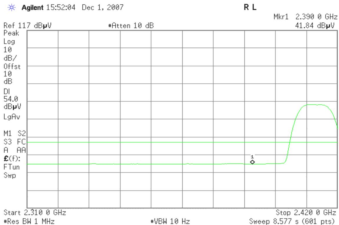
**Band Edges (IEEE 802.11b / CH High)****Detector mode: Peak****Polarity: Vertical**
