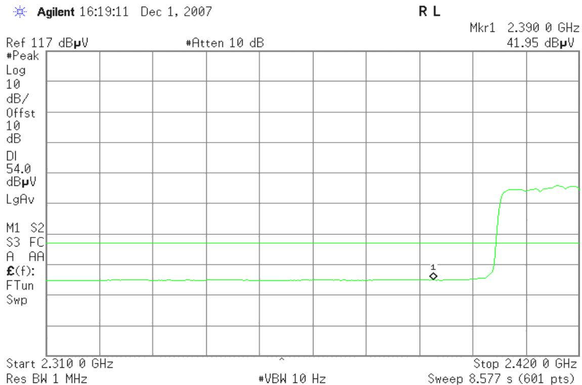
**Band Edges (IEEE 802.11g / CH High)****Detector mode: Peak****Polarity: Vertical**
