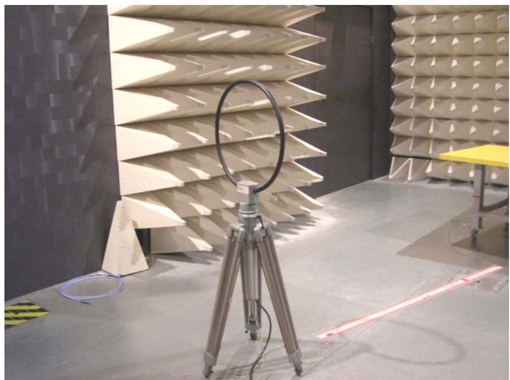
Test Configuration: 30MHz ~ 1GHz
