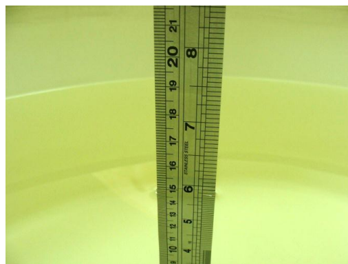
Fig 6.2 Photo of Liquid Height for Body SAR
