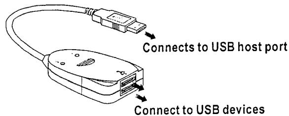
2. Connect USB devices to the Hub: Down 1- Down 2.
