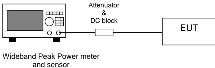
**Note 1:** The EUT was tested while in a continuous transmit mode and the worst case data rates are 1 Mbps for 802.11b, 6 Mbps for 802.11a/ 11g. The EUT was tuned to a low, middle and high channel.
