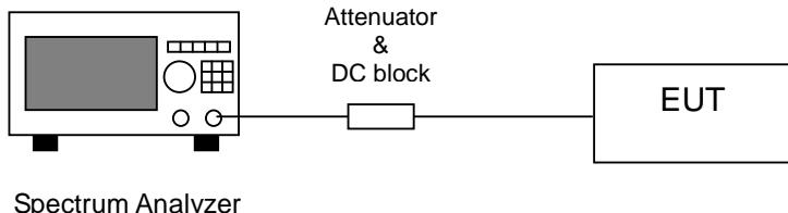
**Note:** The EUT was tested while in a continuous transmit mode and the worst case data rates are 1 Mbps for 802.11b, 6 Mbps for 802.11a/ 11g. The EUT was tuned to a low, middle and high channels with higher power setting.
