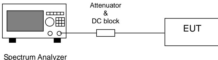
**Note:** The EUT was tested while in a continuous transmit mode and the worst case data rates are 1 Mbps for 802.11b, 6 Mbps for 802.11a/ 11g. The EUT was tuned to a low, middle and high channel.
