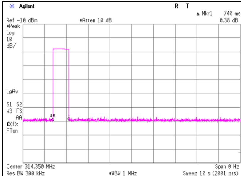
\* The test was performed by a request signal (BLE) from Smart phone operation as representative, because the EUT transmits UHF when LF signal is received from a vehicle or a request signal (BLE) from Smart phone is received, and the UHF transmission is stopped within 5 seconds even when receiving LF signal from vehicle.
