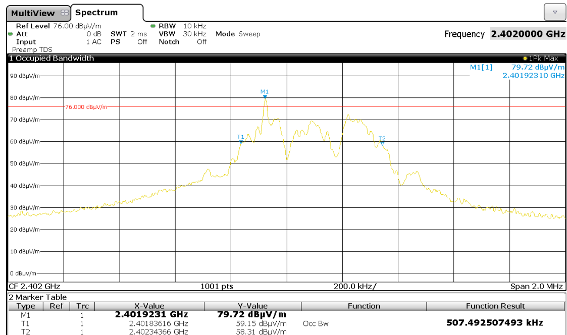
Graph 6-18: Occupied bandwidth – Low channel 2402 MHz
