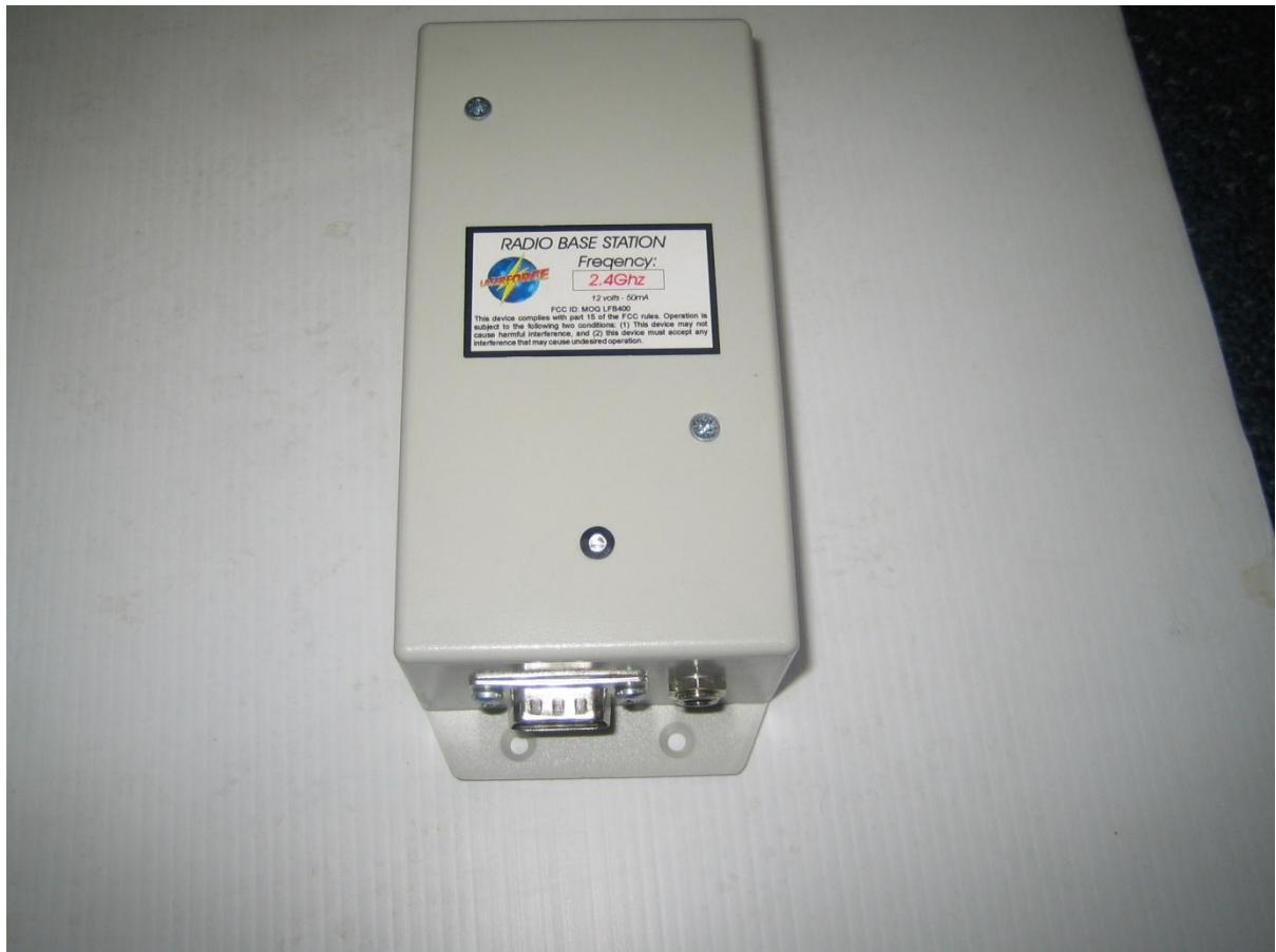
The radio base station in the Gen6 system has a short antenna and operates on a 2.4Ghz frequency, which is the same frequency as wireless networks and some cordless phones. However, the Laserforce system uses complex error checking to filter out any interference with any other equipment. The Laserforce system also does not interfere with other equipment.
