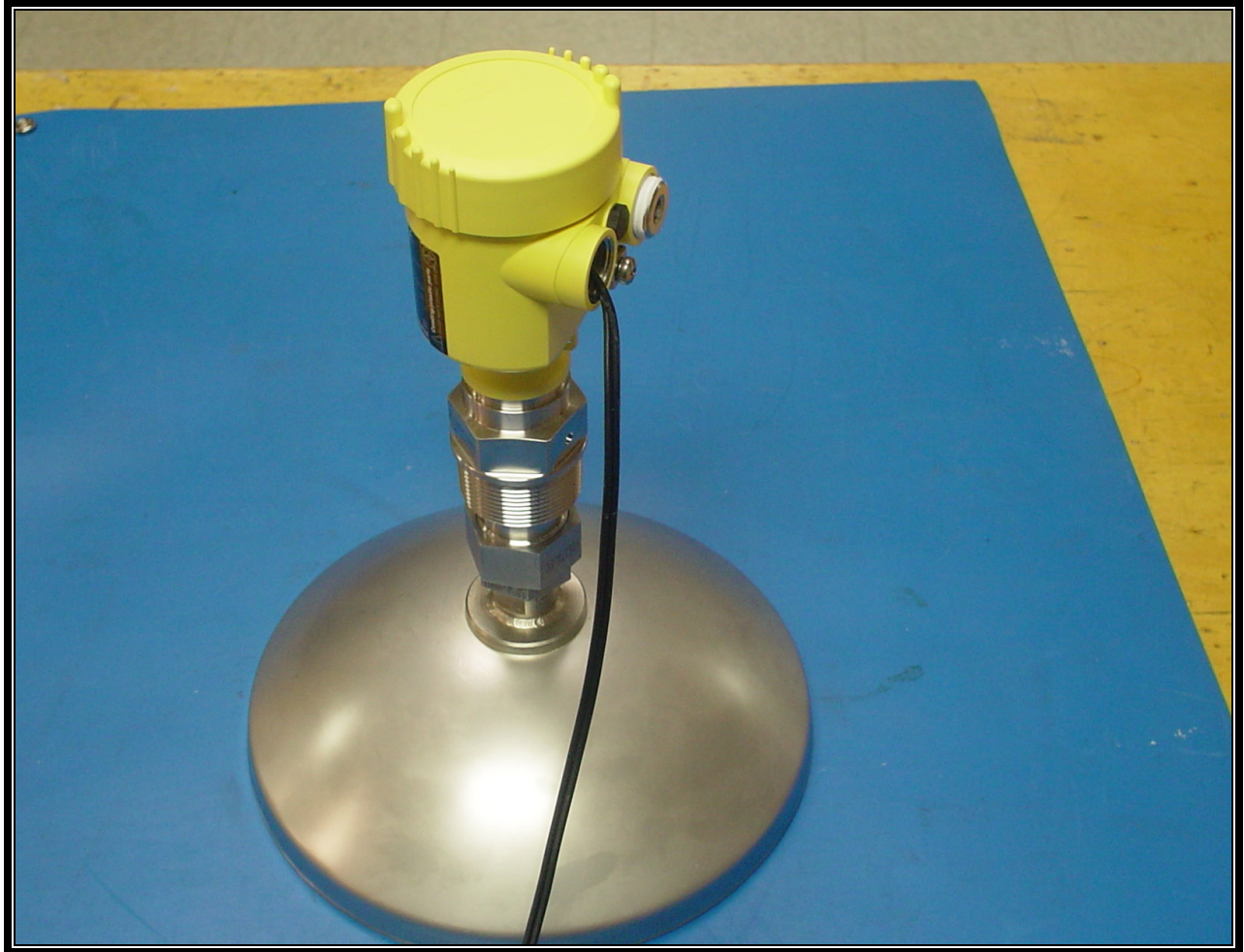
PHOTOGRAPH 5: EUT WITH 33 DBI HORN ANTENNA
