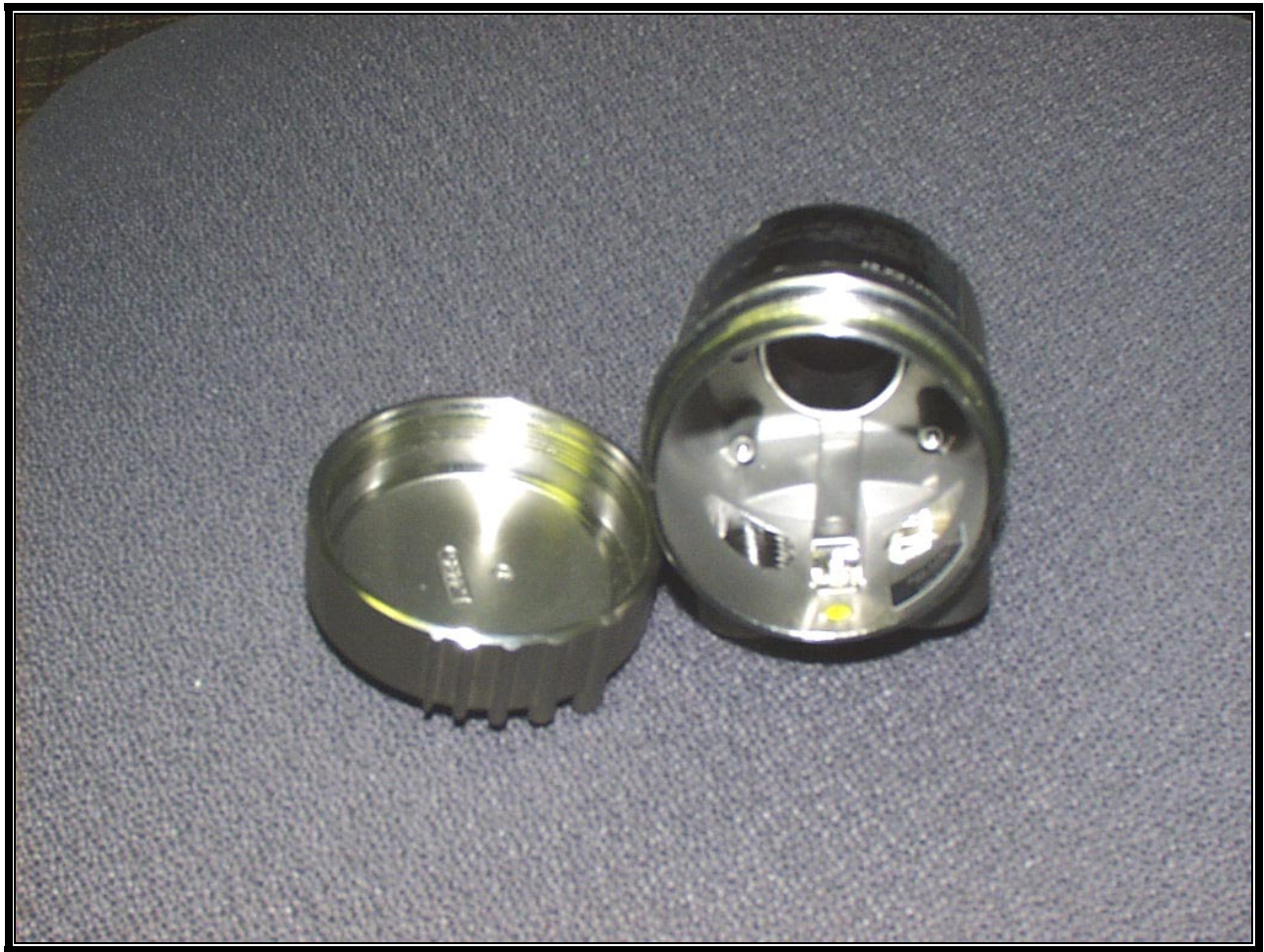
PHOTOGRAPH 14: EUT STAINLESS STEEL HOUSING TOP VIEW
