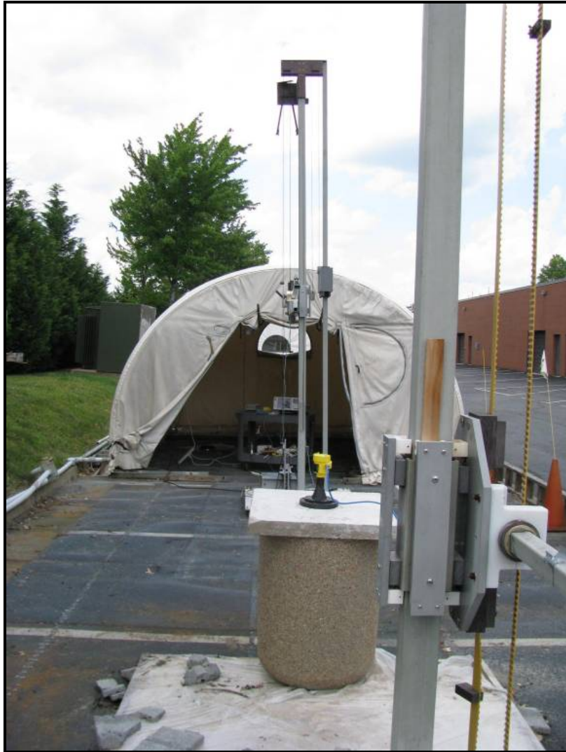
Photograph 3: Radiated Emissions - EUT in Concrete Tank
