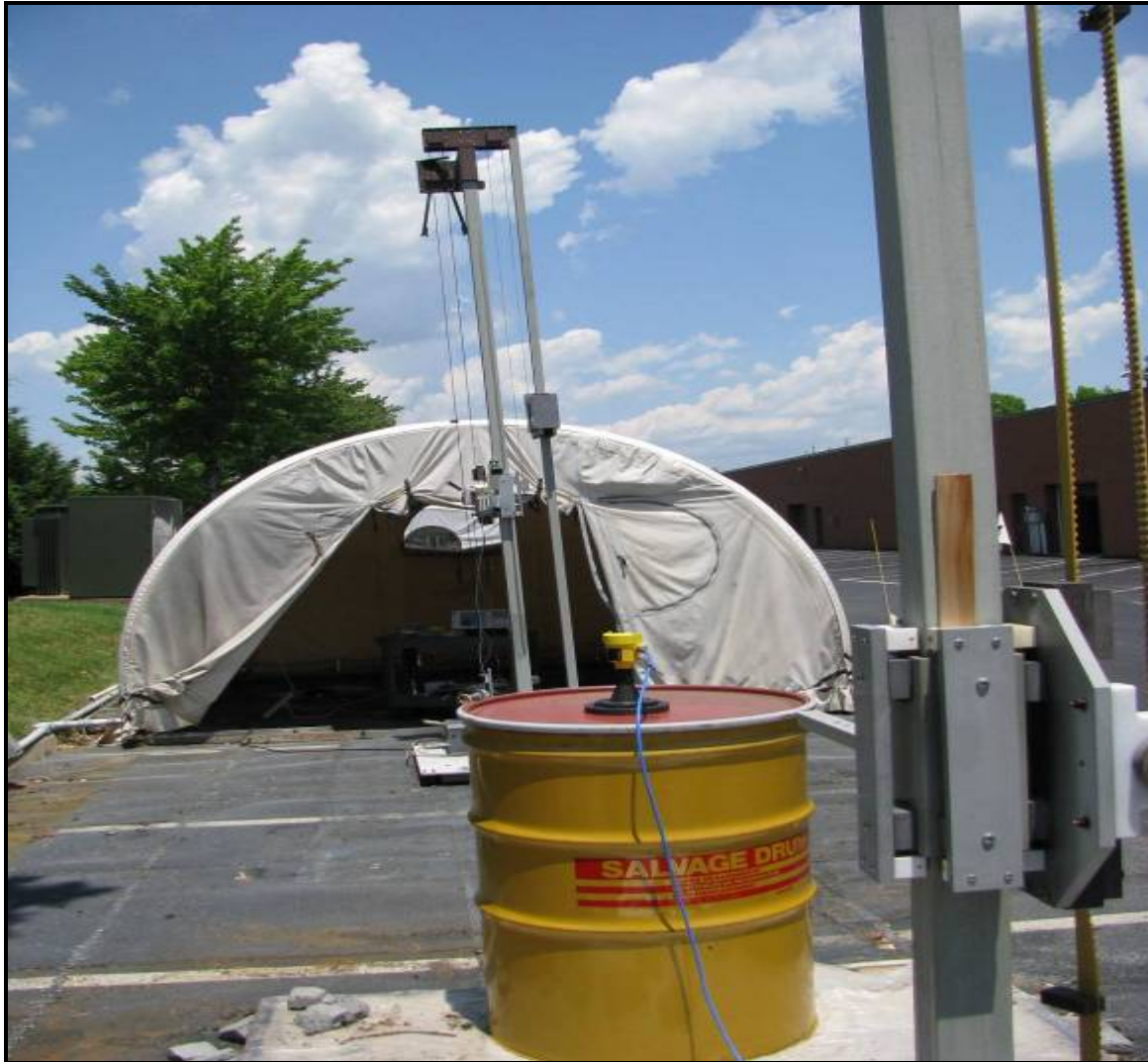
Photograph 2: Radiated Emissions - EUT in Metal Tank
