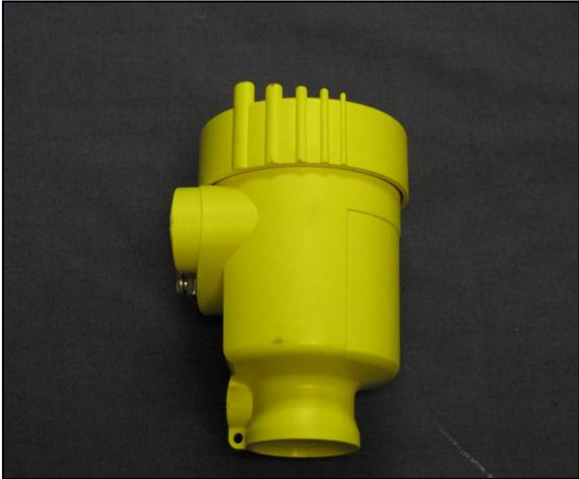
Photograph 10: Plastic Housing with Metalized Inside
