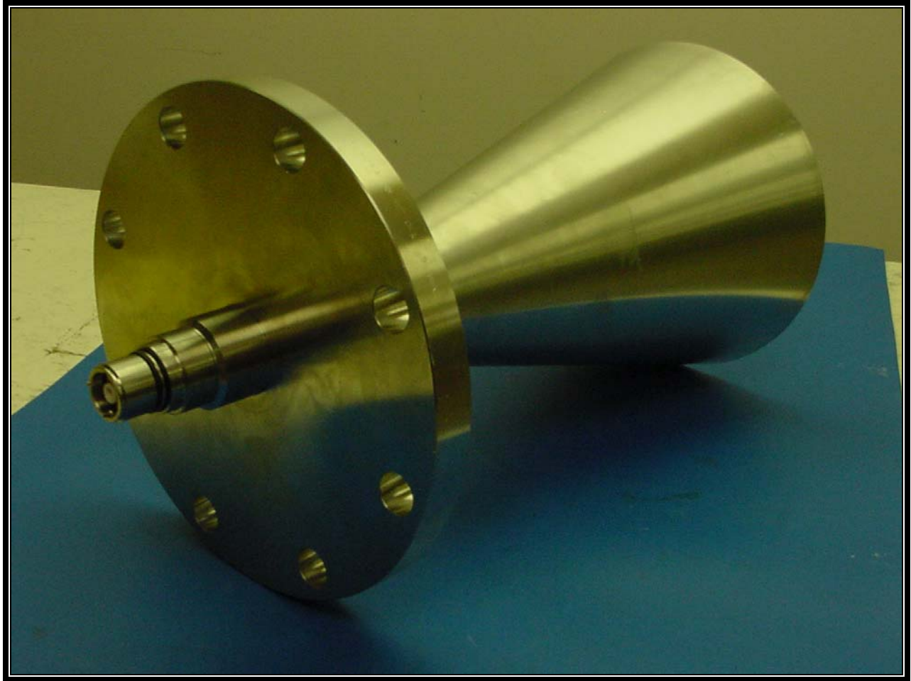
PHOTOGRAPH 24: EUT 21.0 DBI HORN ANTENNA
