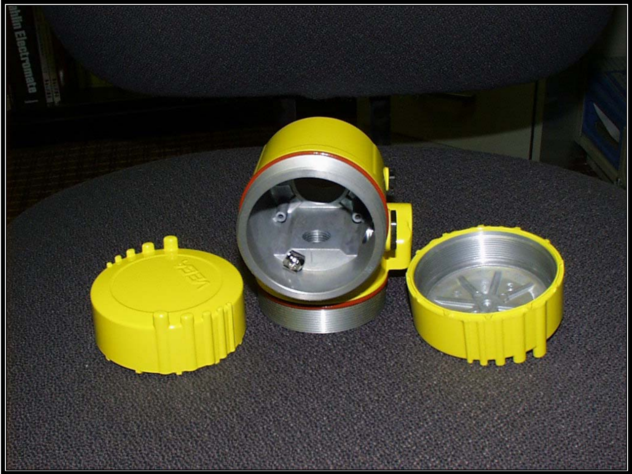
PHOTOGRAPH 14: EUT DOUBLE ALUMINIUM HOUSING FITTING FRONT VIEW
