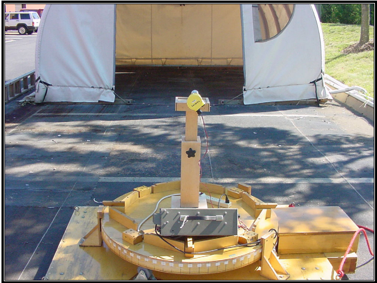
PHOTOGRAPH 3: RADIATED EMISSIONS REAR VIEW 19DBI HORN
