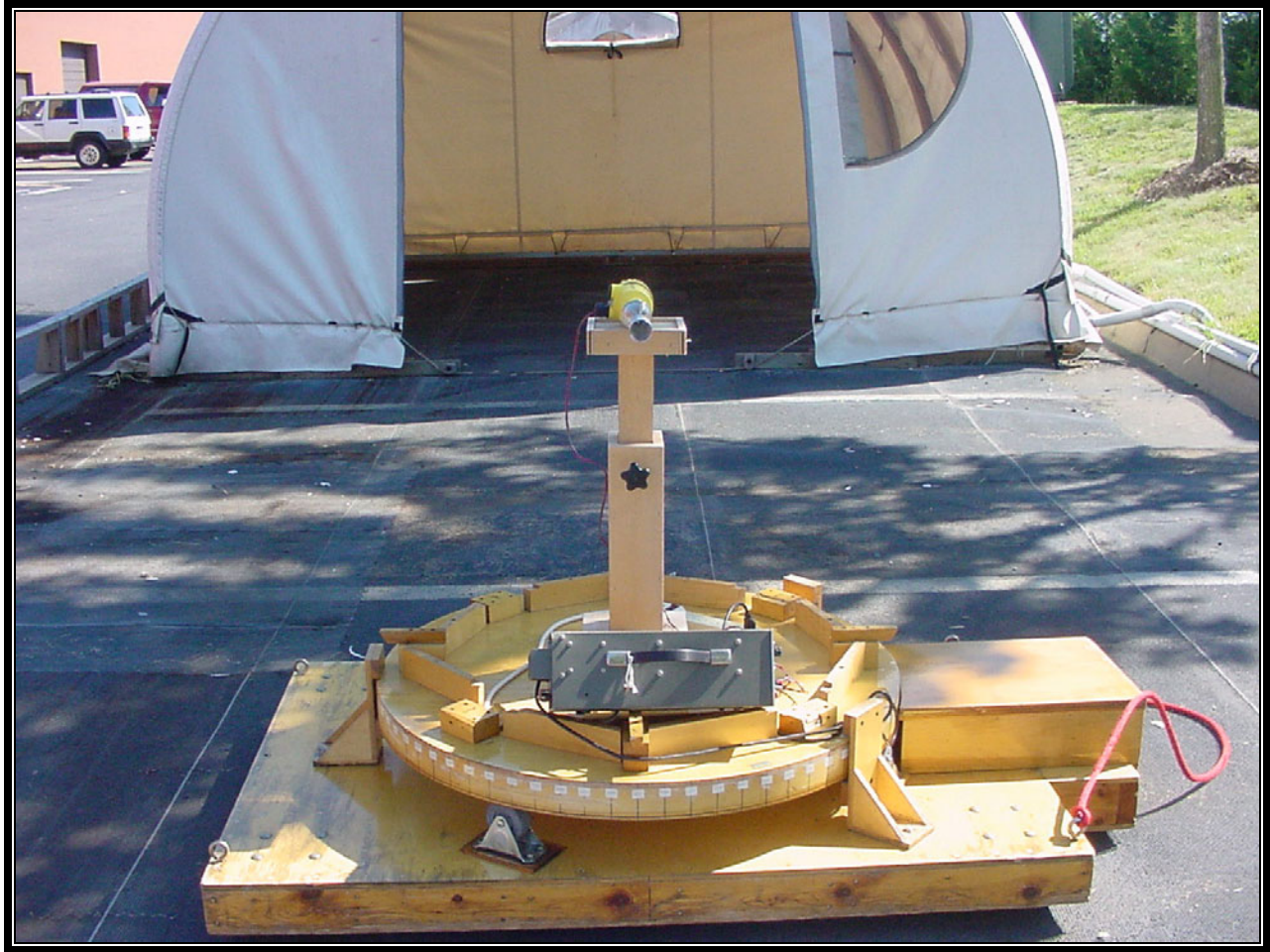
PHOTOGRAPH 2: RADIATED EMISSIONS FRONT VIEW 19DBI HORN
