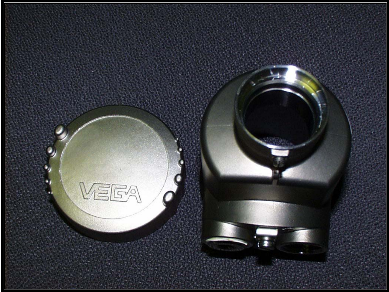
PHOTOGRAPH 18: EUT STAINLESS STEEL HOUSING FITTING
