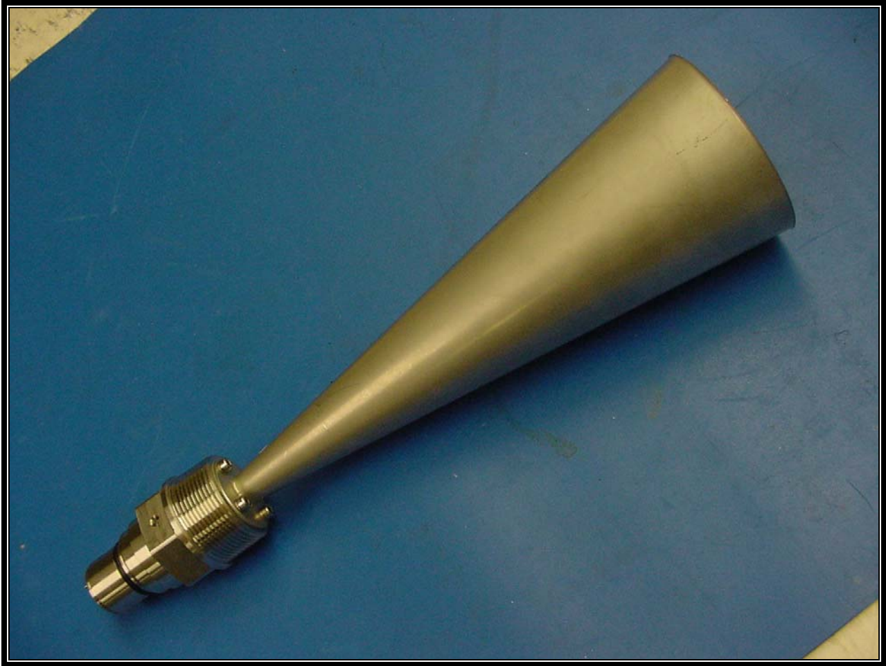
PHOTOGRAPH 28: 24.7 DBI HORN ANTENNA
