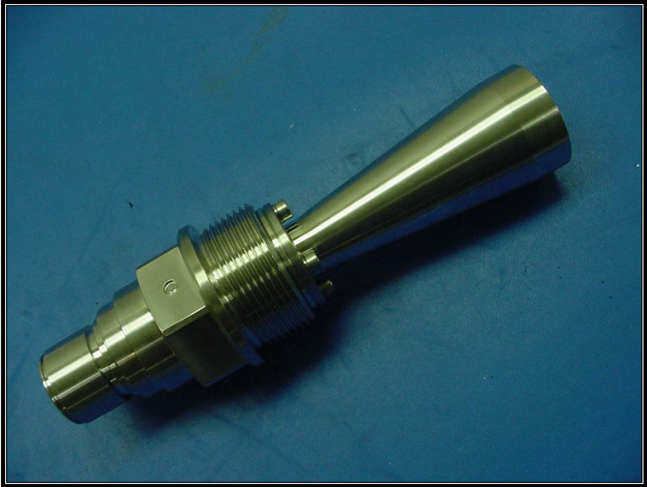
PHOTOGRAPH 22: 19 DBI HORN ANTENNA
