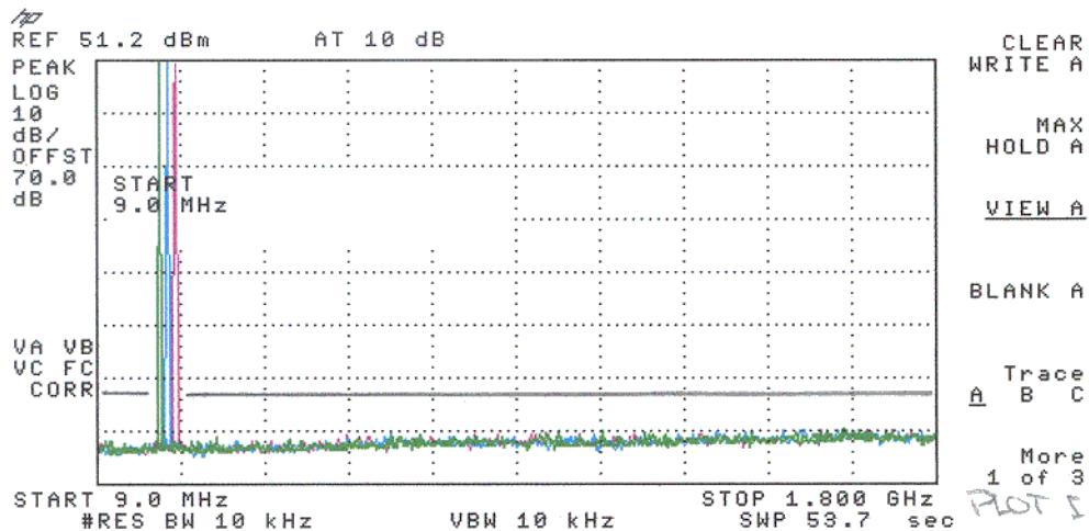
**4.5 FIELD STRENGTH OF RADIATED SPURIOUS EMISSIONS**
