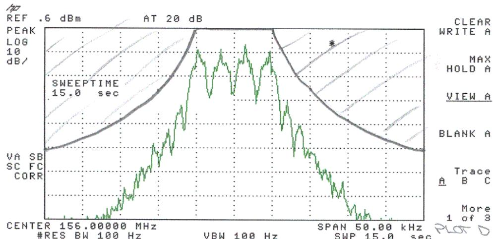
4.3.5 Occupied Bandwidth, 6400 BAUD, ERMES, 4 LEVEL
