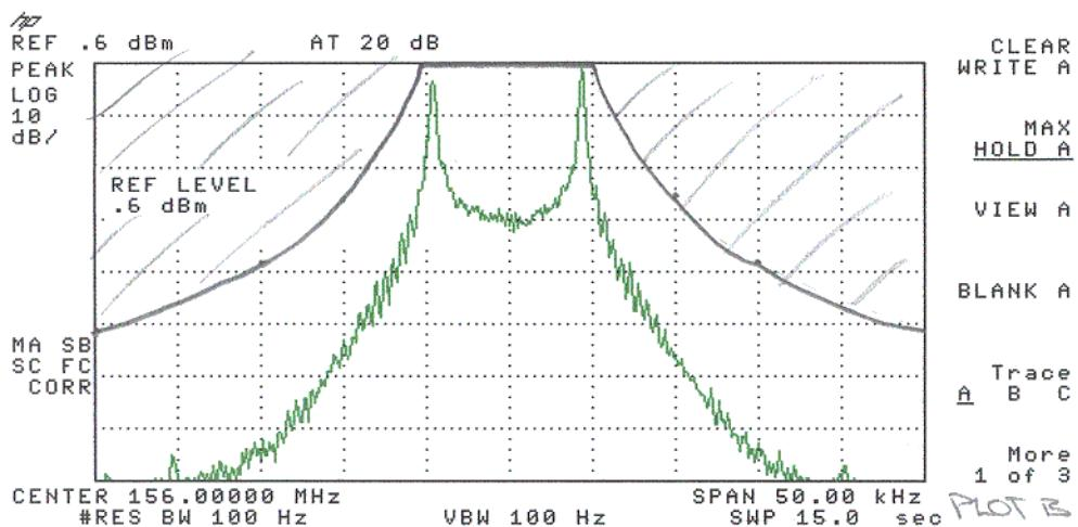
4.3.3 Occupied Bandwidth, 2400 BAUD, POCSAG
