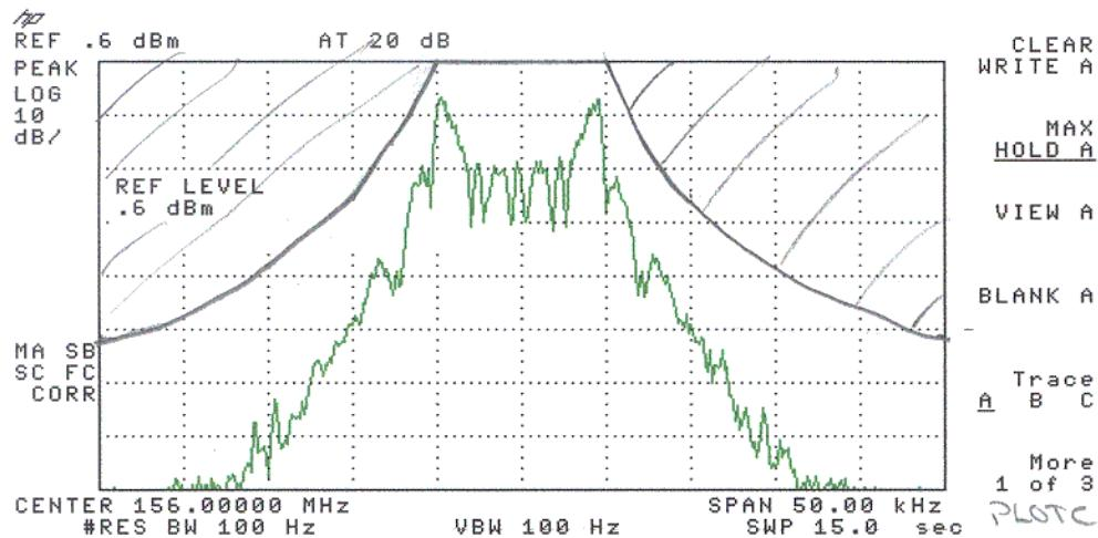
4.3.4 Occupied Channel Bandwidth 3200 BAUD, ERMES, 4-LEVEL
