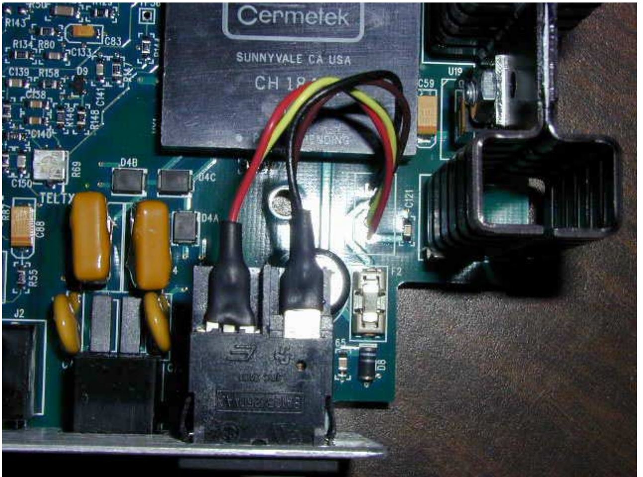
Main board switch inserted
