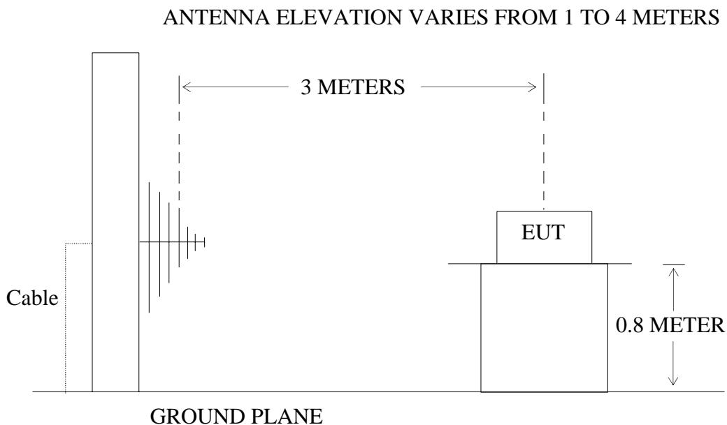
(EUT: Wireless Stereo Speaker System Transmitter)
