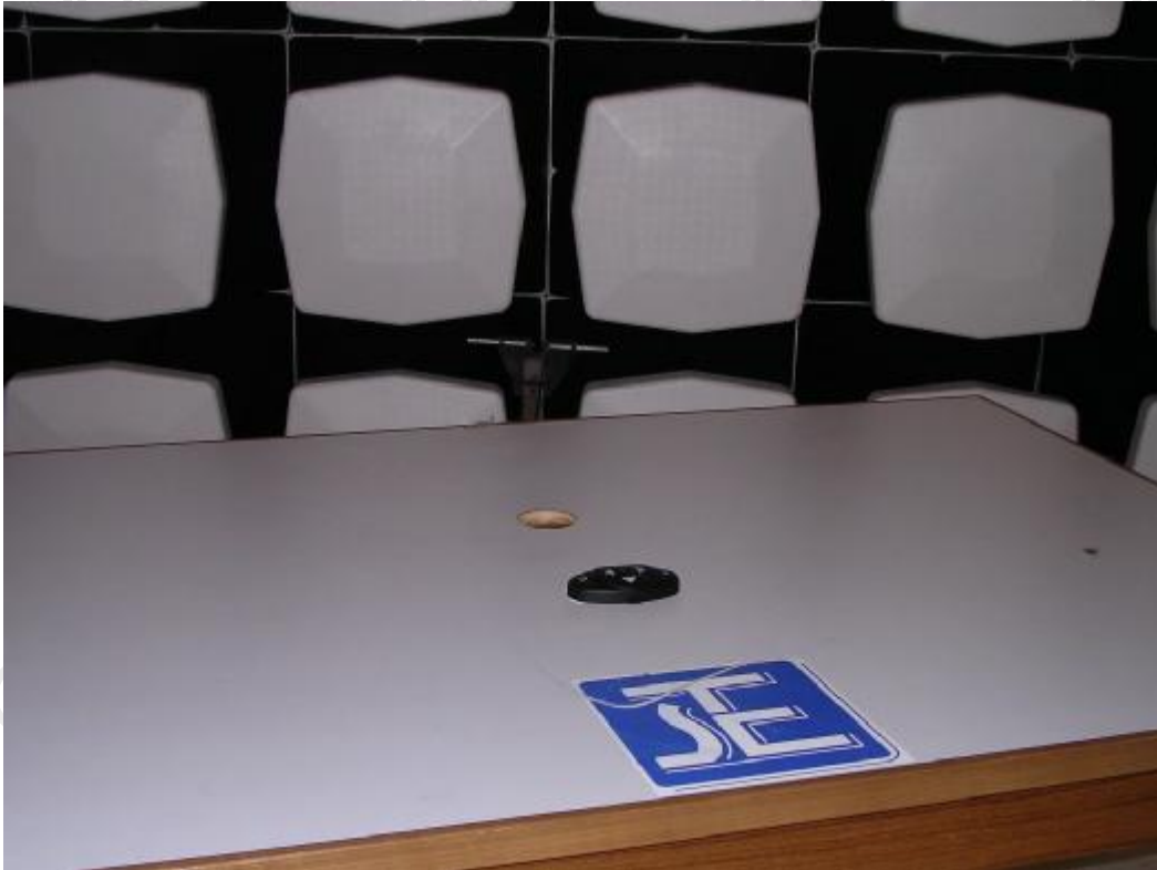
Measurement of Radiated Emission Test Set Up
