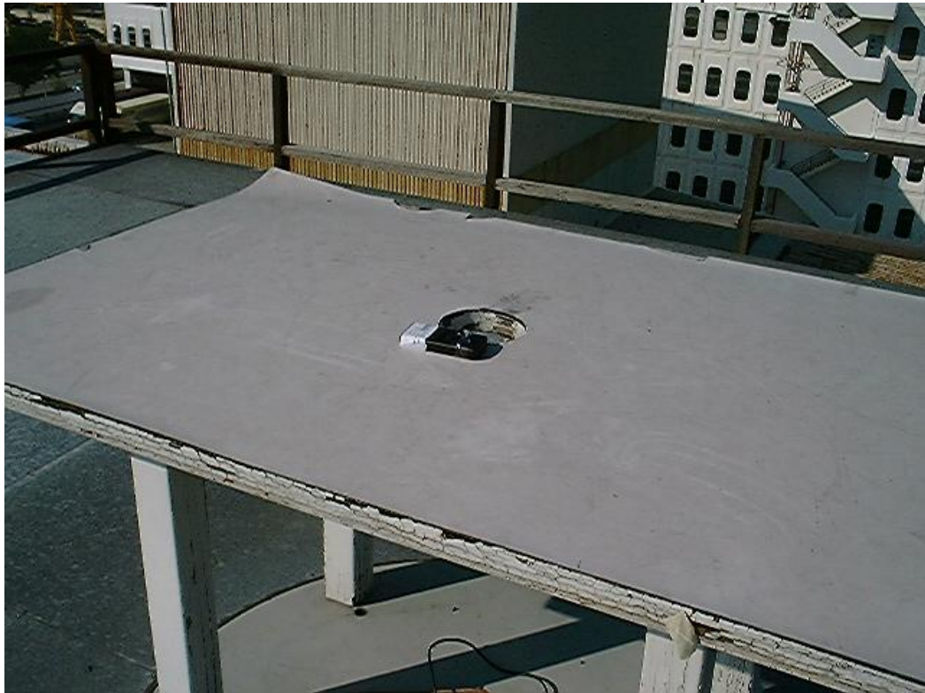
Measurement of Radiated Emission Test Set Up
