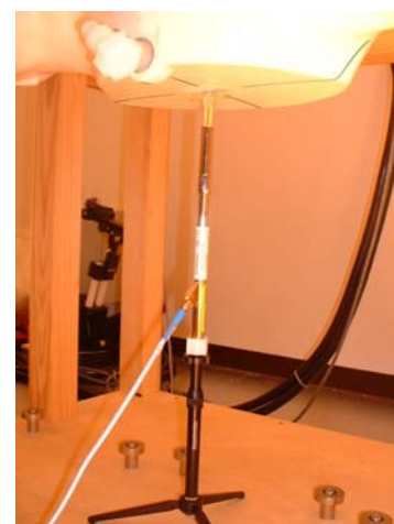
2450MHz System performance check setup
