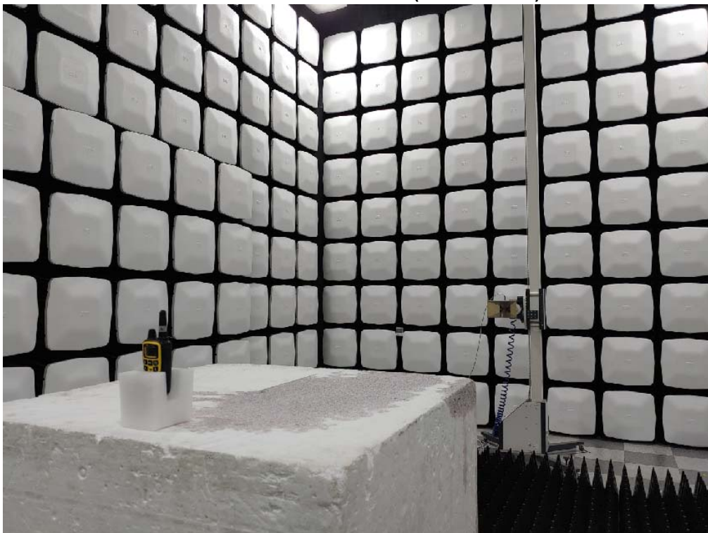
Radiated RF measurement(Above 1 GHz)
