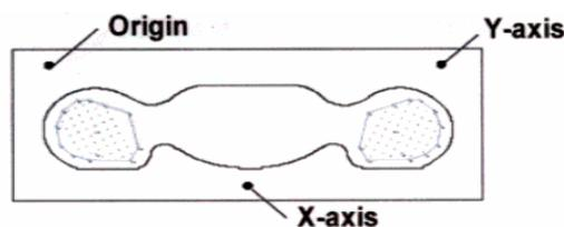
Fig. 10. SAR Measurement Point in Area Scan
