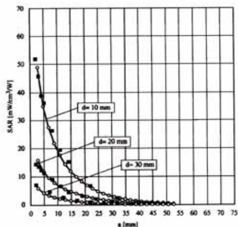
Figure 7. E-Field and temperature measurements at 1.8GHz [5]
