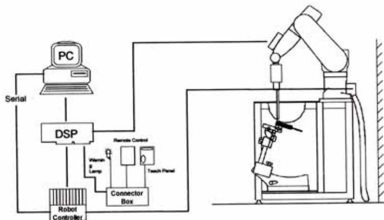
Figure 3. HCT SAR Lab. Test Measurement Set-up
