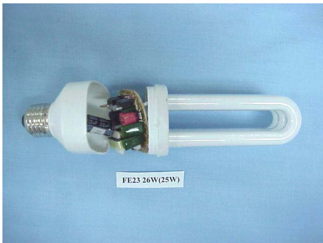
FIGURE 7 ENERGY SAVING LAMP (M/N: FE23 26W(25W)) COVER REMOVED
