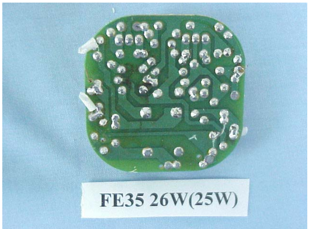
FIGURE 36 ENERGY SAVING LAMP (M/N: FE35 26W(25W)) MAIN BOARD (SOLDERED SIDE)
