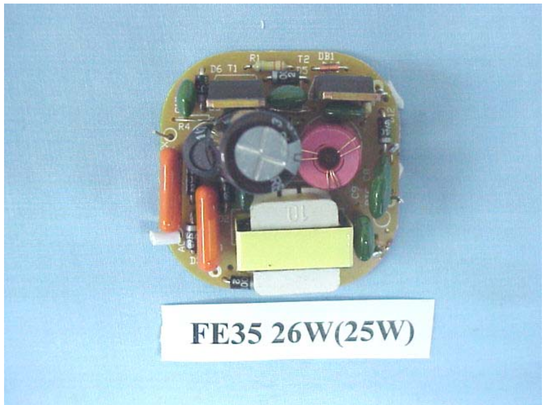
FIGURE 35 ENERGY SAVING LAMP (M/N: FE35 26W(25W)) MAIN BOARD (COMPONENT SIDE)
