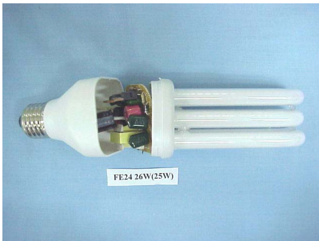
FIGURE 16 ENERGY SAVING LAMP (M/N: FE24 26W(25W)) COVER REMOVED
