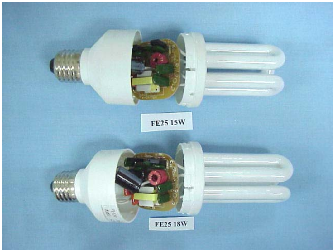
FIGURE 19 ENERGY SAVING LAMP (M/N: FE25 15W/18W) COVER REMOVED
