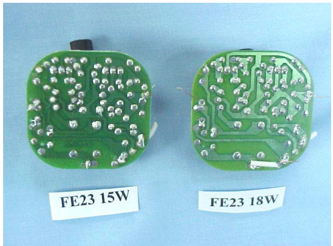
FIGURE 3 ENERGY SAVING LAMP (M/N: FE23 15W/18W) MAIN BOARD (SOLDERED SIDE)
