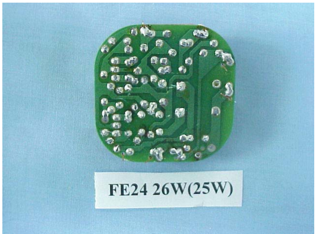
FIGURE 18 ENERGY SAVING LAMP (M/N: FE24 26W(25W)) MAIN BOARD (SOLDERED SIDE)
