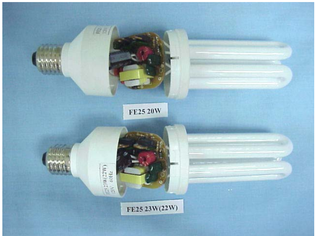
FIGURE 22 ENERGY SAVING LAMP (M/N: FE25 20W/23W(22W)) COVER REMOVED
