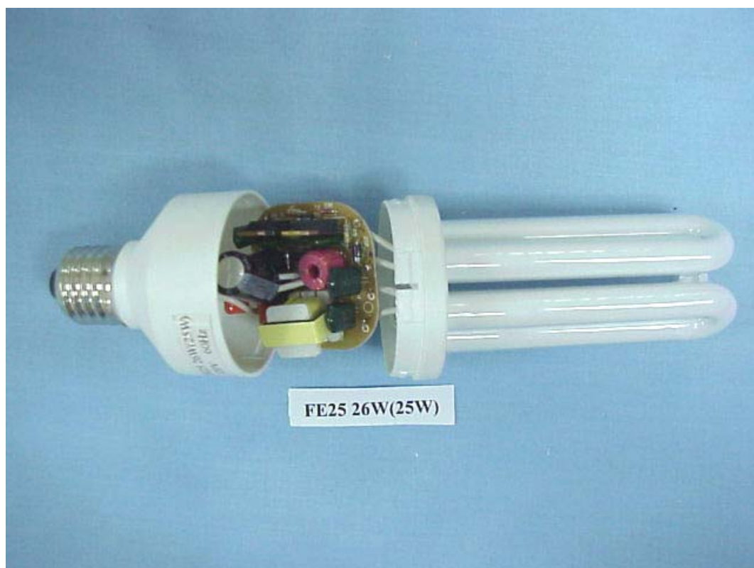
FIGURE 25 ENERGY SAVING LAMP (M/N: FE25 26W(25W)) COVER REMOVED
