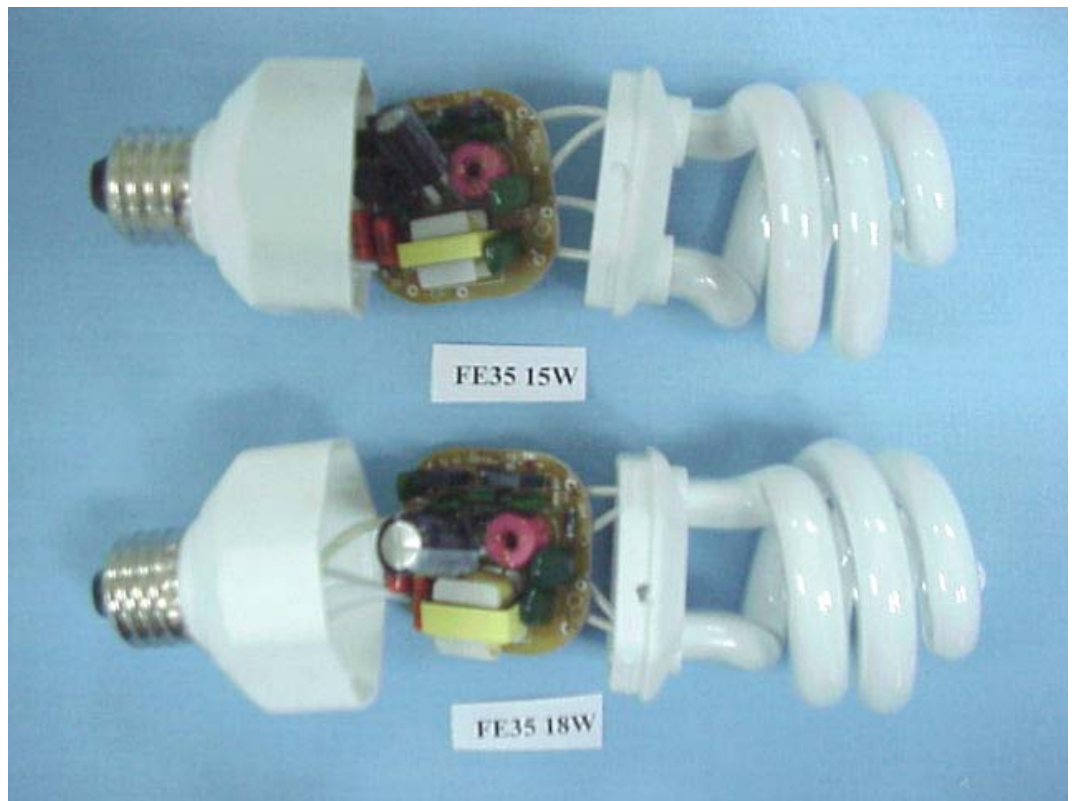
FIGURE 28 ENERGY SAVING LAMP (M/N: FE35 15W/18W) COVER REMOVED
