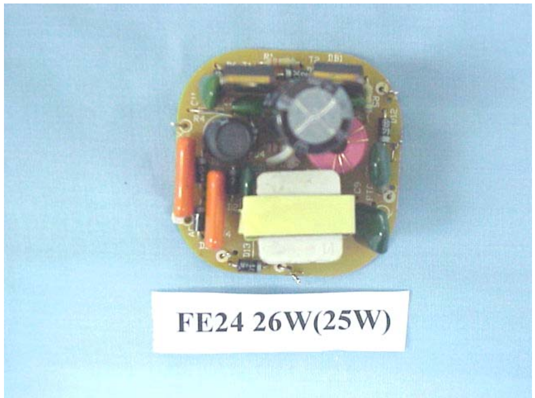
FIGURE 17 ENERGY SAVING LAMP (M/N: FE24 26W(25W)) MAIN BOARD (COMPONENT SIDE)
