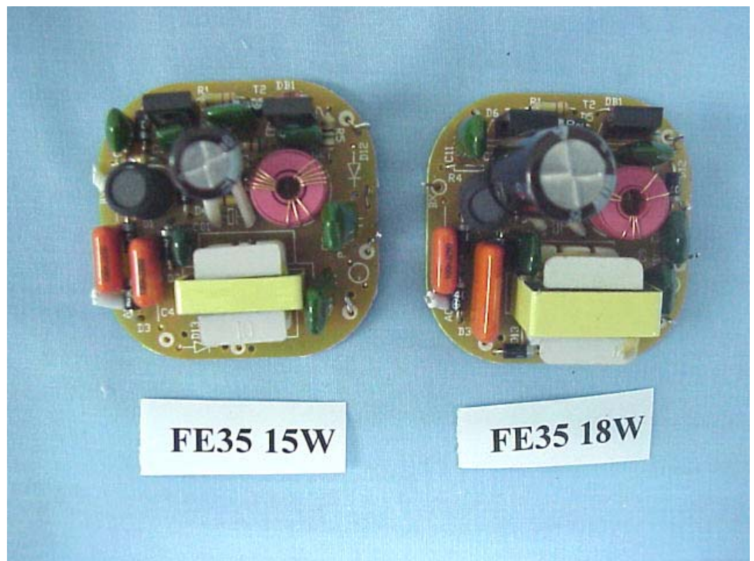
FIGURE 29 ENERGY SAVING LAMP (M/N: FE35 15W/18W) MAIN BOARD (COMPONENT SIDE)
