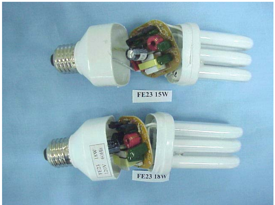
FIGURE 1 ENERGY SAVING LAMP (M/N: FE23 15W/18W) COVER REMOVED
