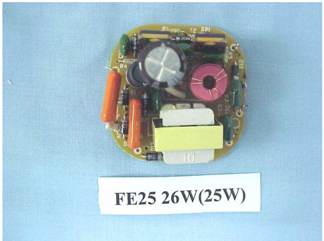
FIGURE 26 ENERGY SAVING LAMP (M/N: FE25 26W(25W)) MAIN BOARD (COMPONENT SIDE)
