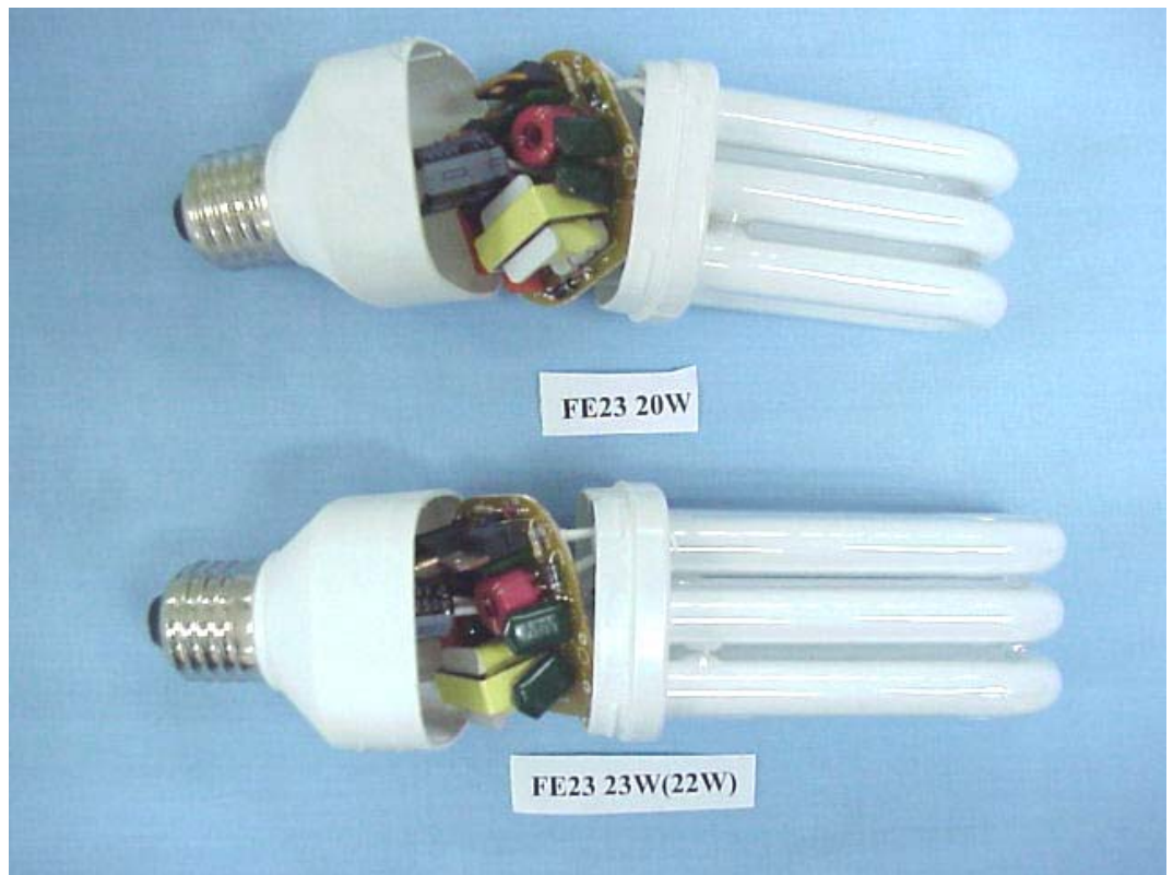
FIGURE 4 ENERGY SAVING LAMP (M/N: FE23 20W/23W(22W)) COVER REMOVED
