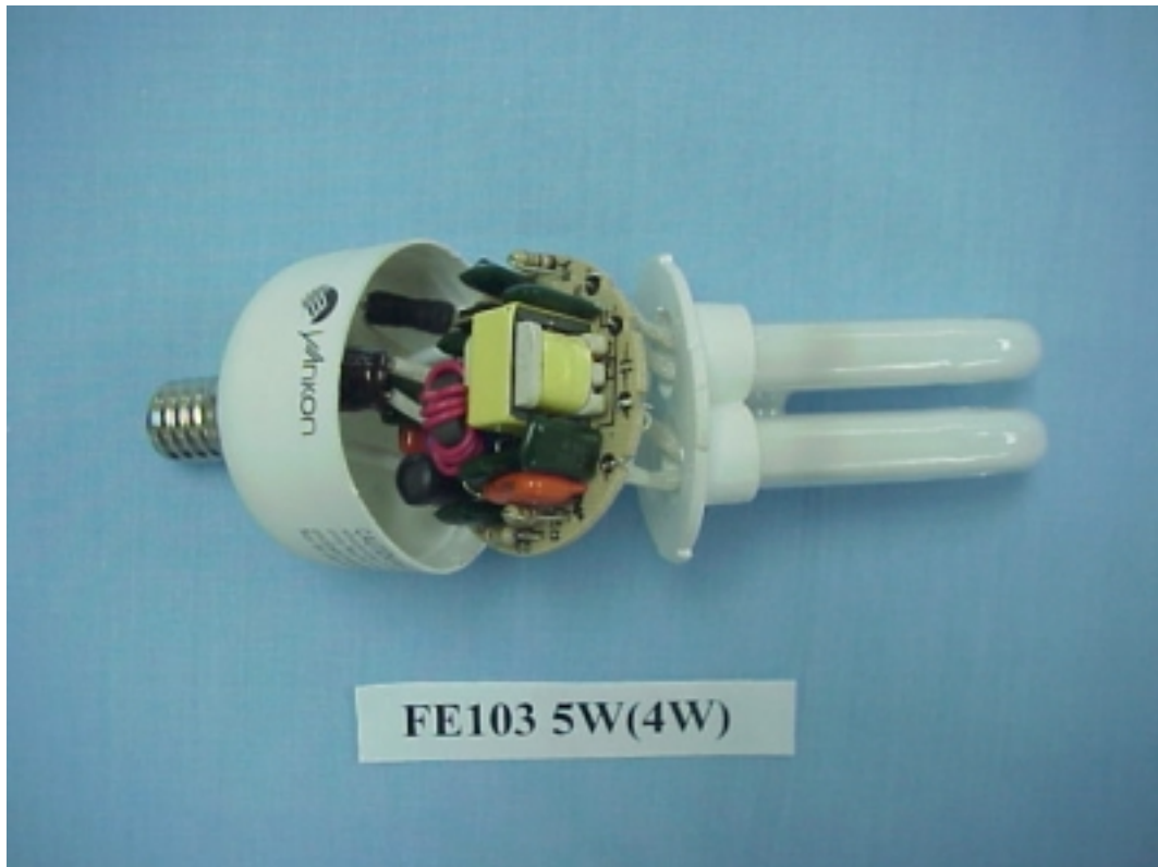
FIGURE 1 ENERGY SAVING LAMP (M/N: FE103 5W(4W)) COVER REMOVED
