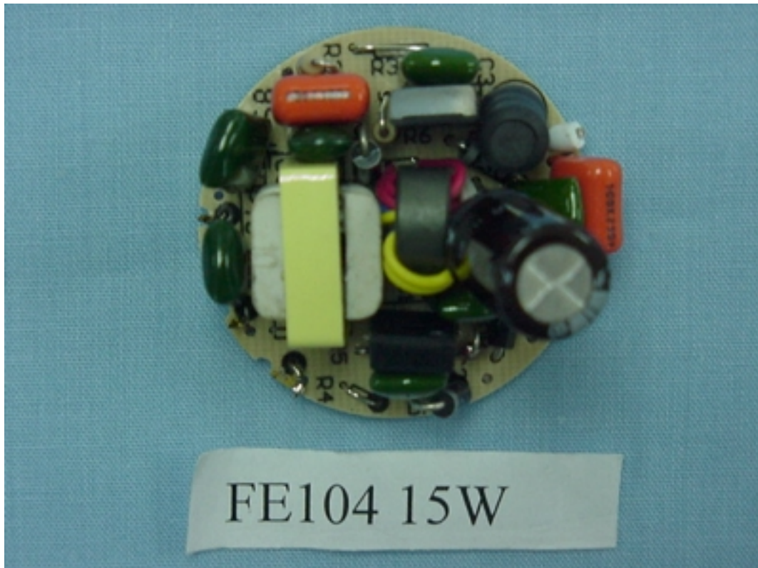
FIGURE 11 ENERGY SAVING LAMP (M/N: FE104 15W) MAIN BOARD (COMPONENT SIDE)
