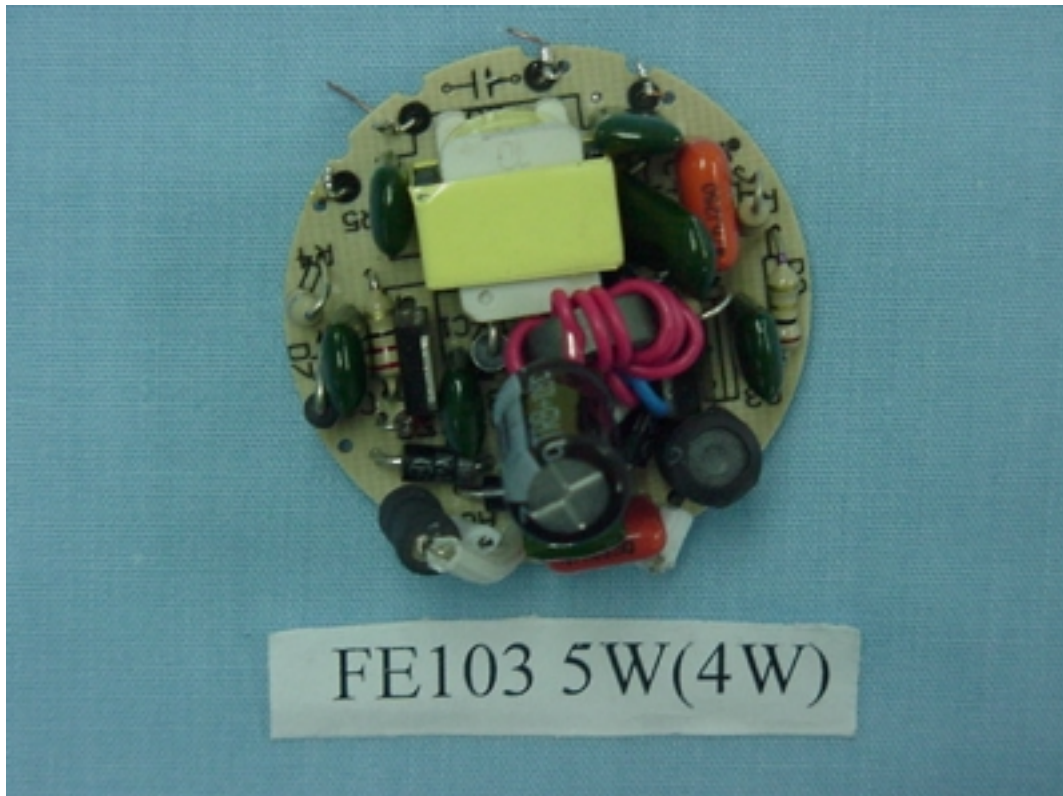
FIGURE 2 ENERGY SAVING LAMP (M/N: FE103 5W(4W)) MAIN BOARD (COMPONENT SIDE)
