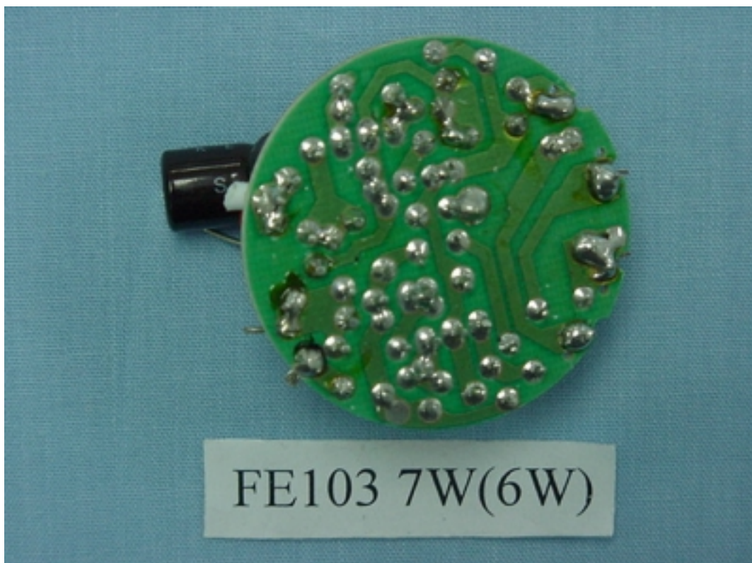
FIGURE 6 ENERGY SAVING LAMP (M/N: FE103 7W(6W)) MAIN BOARD (SOLDERED SIDE)
