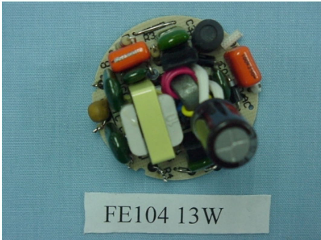
Figure 8 ENERGY SAVING LAMP (M/N: FE104 13W) MAIN BOARD (COMPONENT SIDE)
