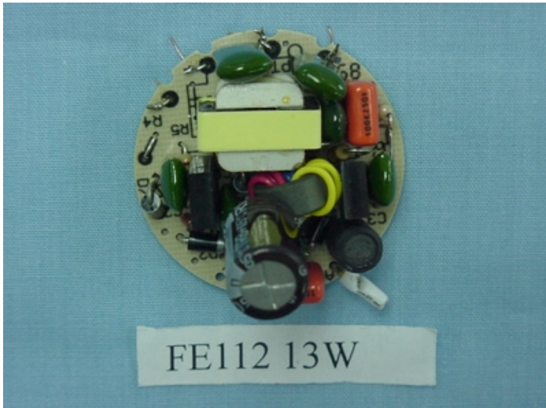
FIGURE 17 ENERGY SAVING LAMP (M/N: FE112 13W) MAIN BOARD (COMPONENT SIDE)
