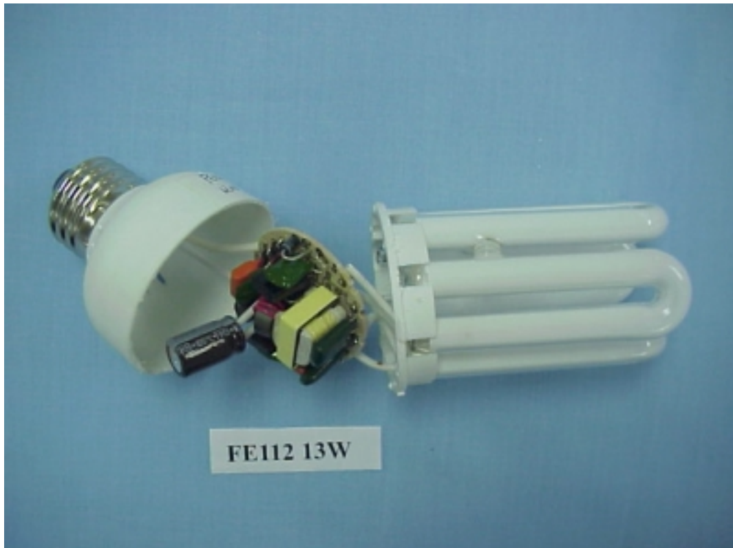
Figure 16 ENERGY SAVING LAMP (M/N: FE112 13W) COVER REMOVED
