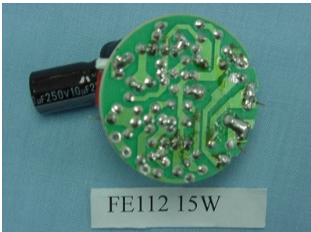
FIGURE 21 ENERGY SAVING LAMP (M/N: FE112 15W) MAIN BOARD (SOLDERED SIDE)
