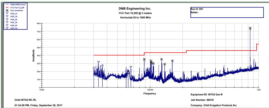
This test is required for any spurious emission or modulation product that falls in a Restricted Band, as defined in Section 15.205. It must be performed with the highest gain of each type of antenna proposed for use with the EUT. Use the following spectrum analyzer settings:
