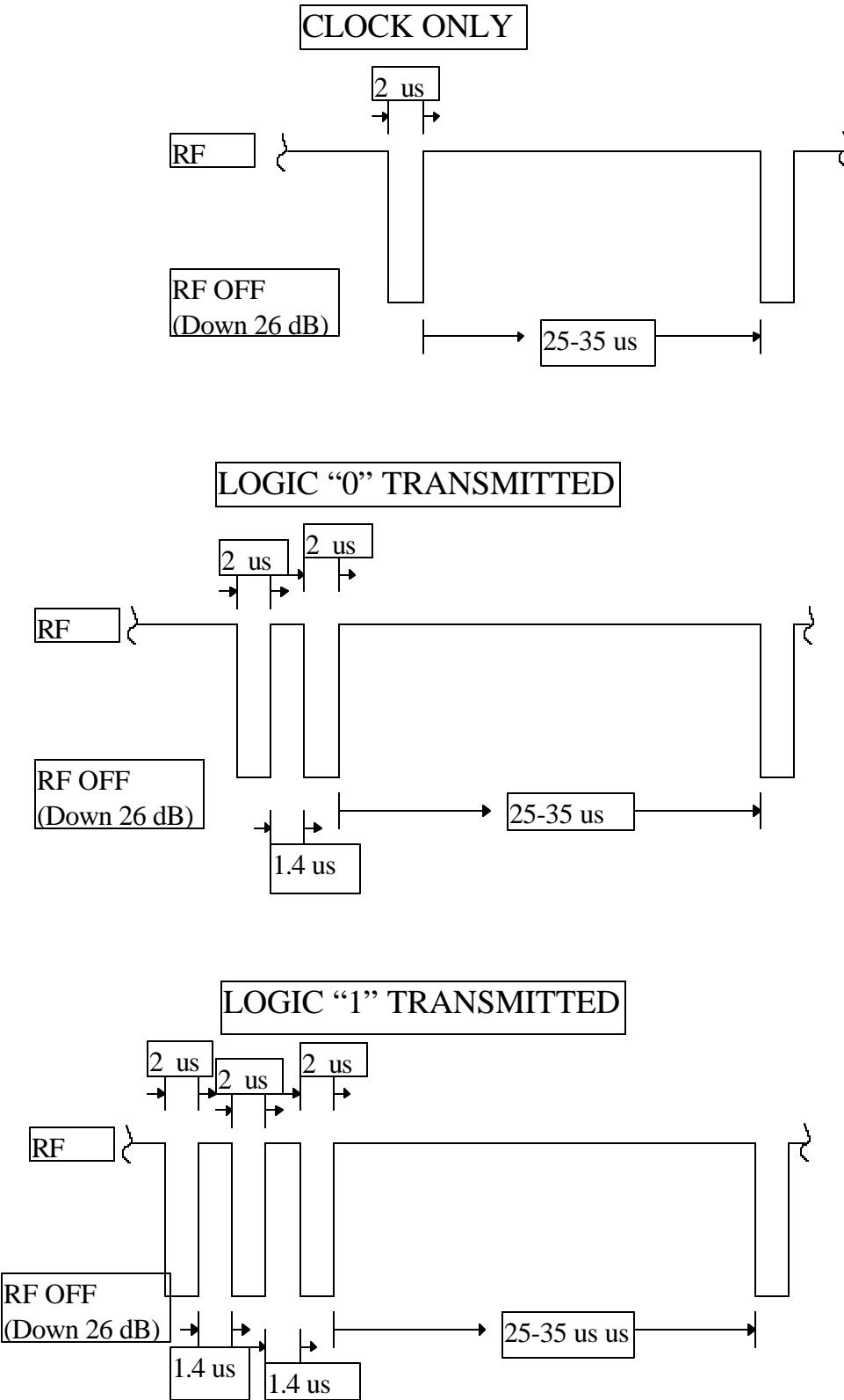
Figure 1 Modulation Modes of the MKRU519 Transceiver
