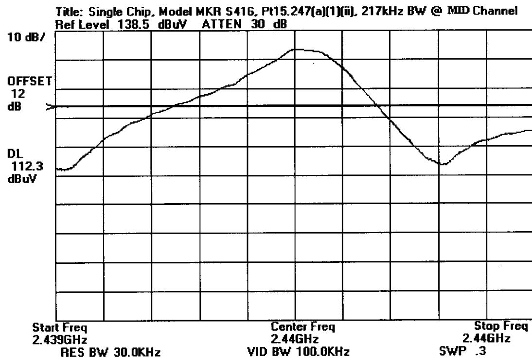
Note: The display line on the plot is 20dBc.
