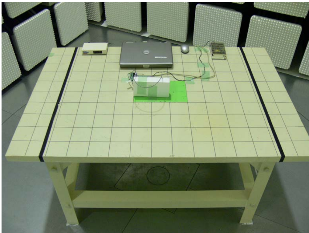
Photograph 15: Set-up for Radiated Emission of Transmitter, Front View
