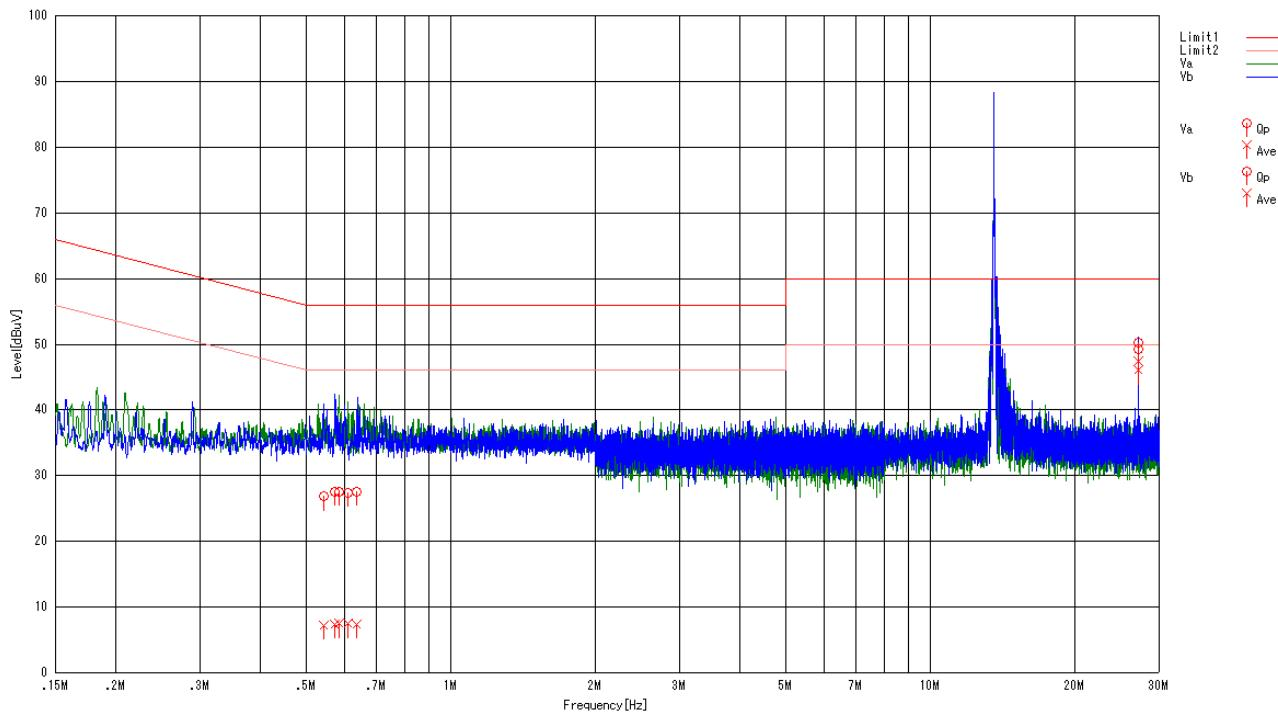
**AC Power line conducted emission. (with dummy load)**
