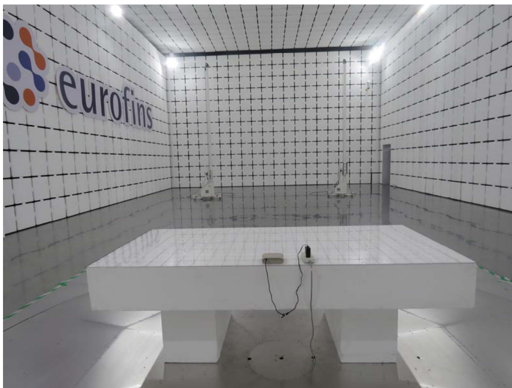
Picture 1: Radiated Emission Test Setup
