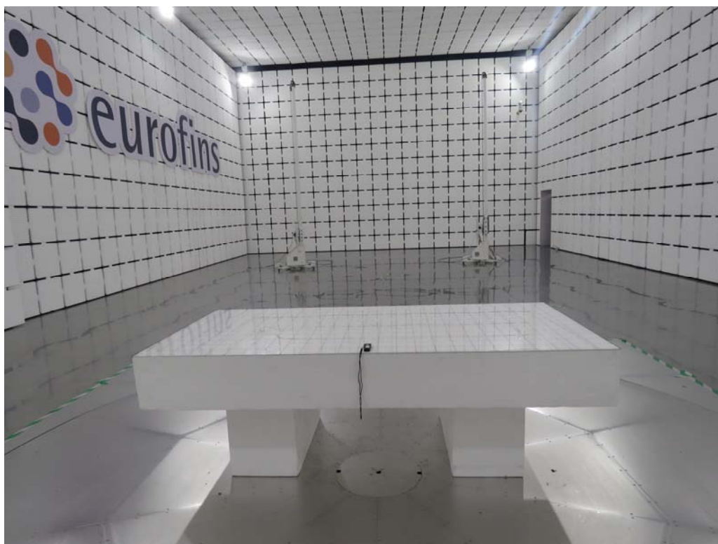
Picture 1: Radiated Emission Test Setup
