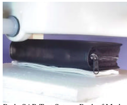
Body SAR Test Setup - Back of Modem (Portfolio Case Closed - Left Side - 1.0cm Separation)
