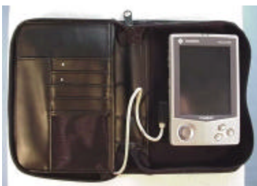
Portfolio Open with PDA (Modem Inside Left Cover of Portfolio Case)
