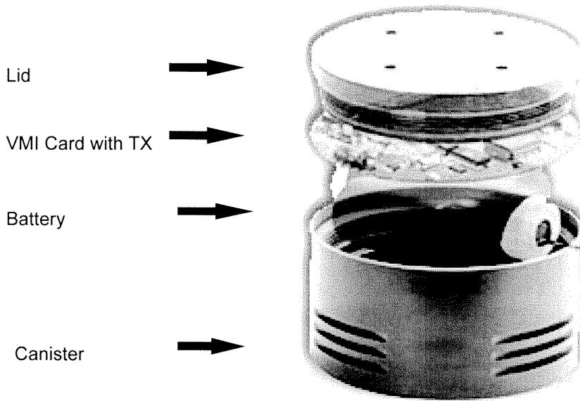
**Canister and Lid:** Molybdenum disulfide filled nylon thermoplastic material machined with wall thickness of 0.6 in, overall diameter is 6 in. Lid is threaded and uses two silicon o-rings to build a water tight seal.
