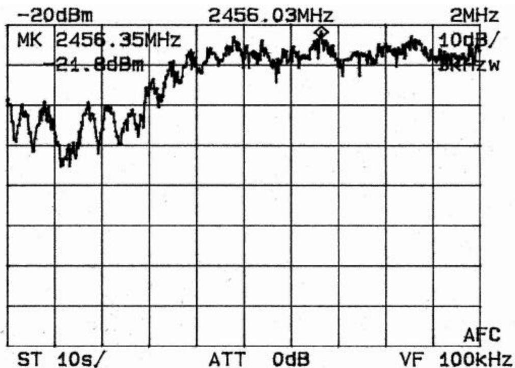
**4.4 FCC Part 15.247(c) Conducted Spurious, 2451 MHz Frequency Of Carrier:**
