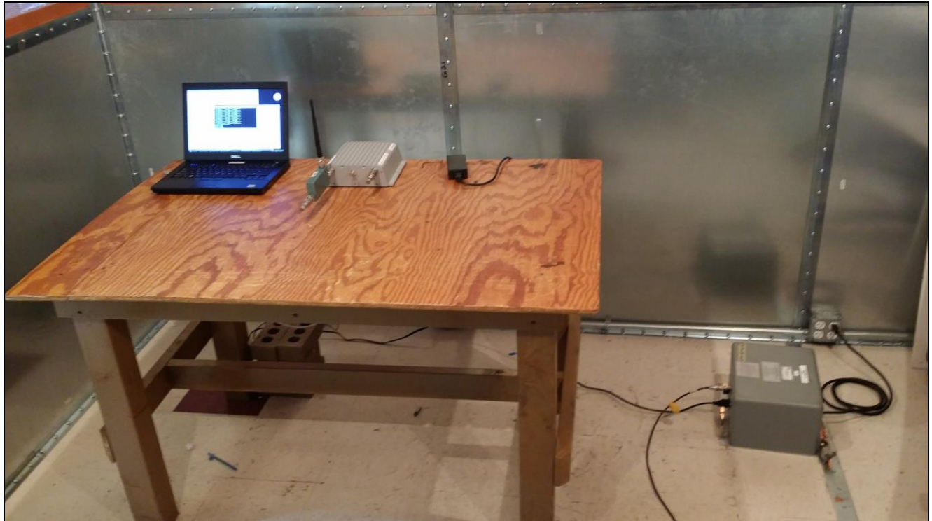
Photograph 4. Conducted Emissions, Test Setup
