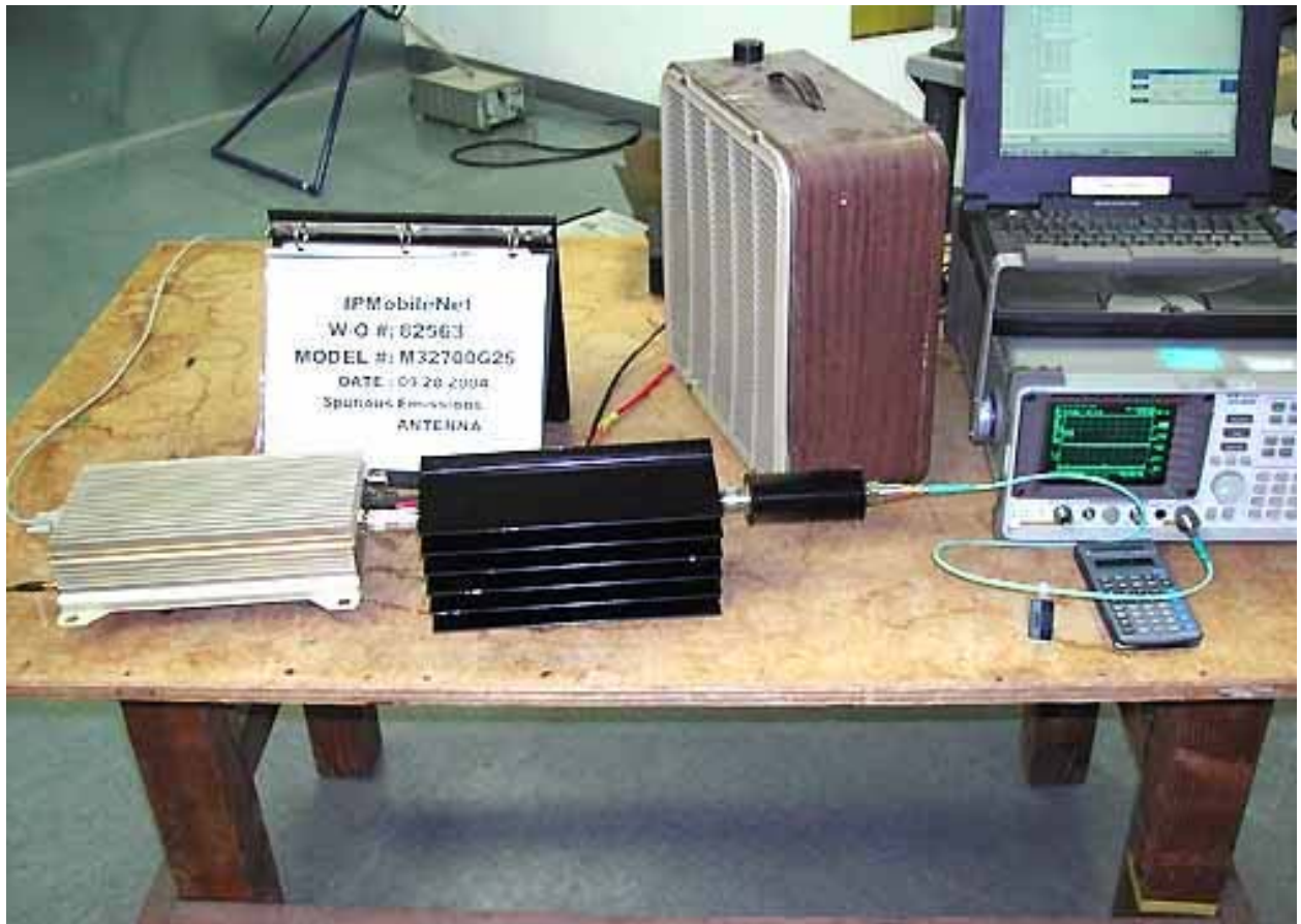
PHOTOGRAPH SHOWING DIRECT CONNECT TEST SETUP
