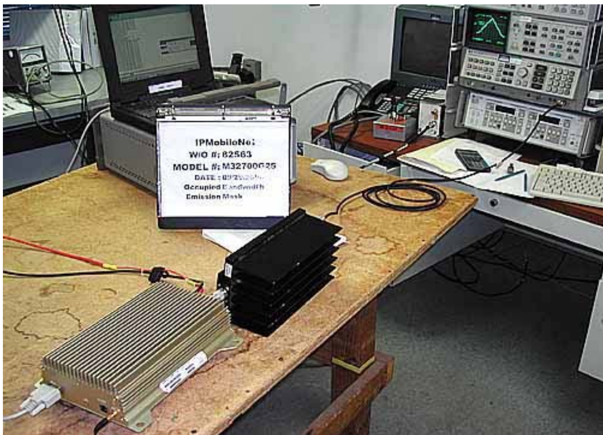
PHOTOGRAPH SHOWING EMISSIONS MASK
