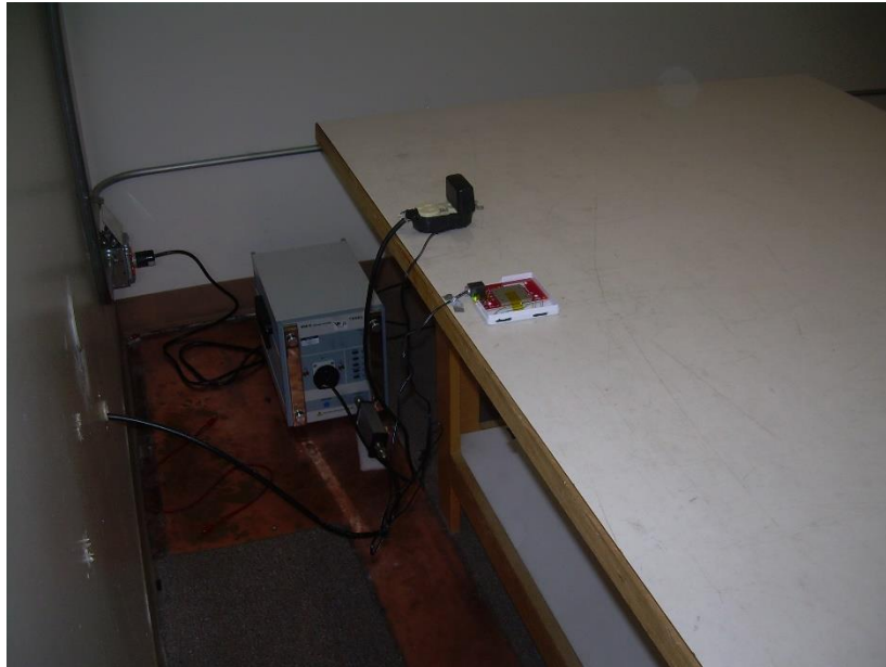
Photograph 5: Back View Conducted Emissions Worst-Case Configuration
