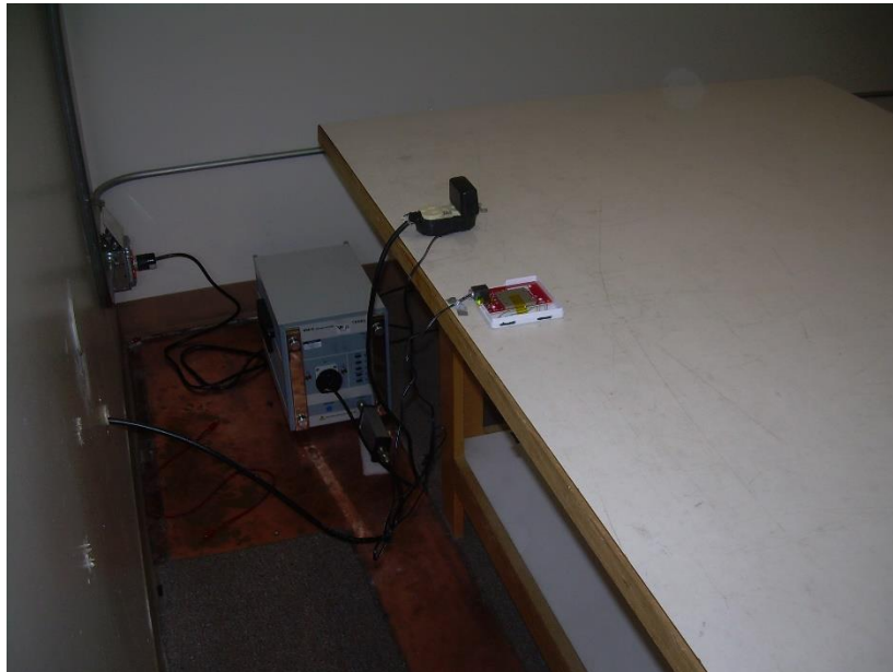
Photograph 8: Back View Conducted Emissions Worst-Case Configuration
