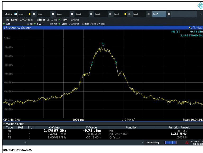
Figure 5 - High Channel (2480 MHz 1M) 20 dB Bandwidth
