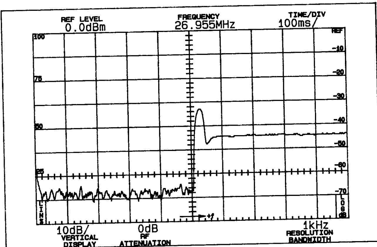
Measurement Conditions: 16 dB over 50% modulation level at 1292 Hz with 2500 Hz tone, lower fourth order sideband; horizontal scale 100 ms/div.
