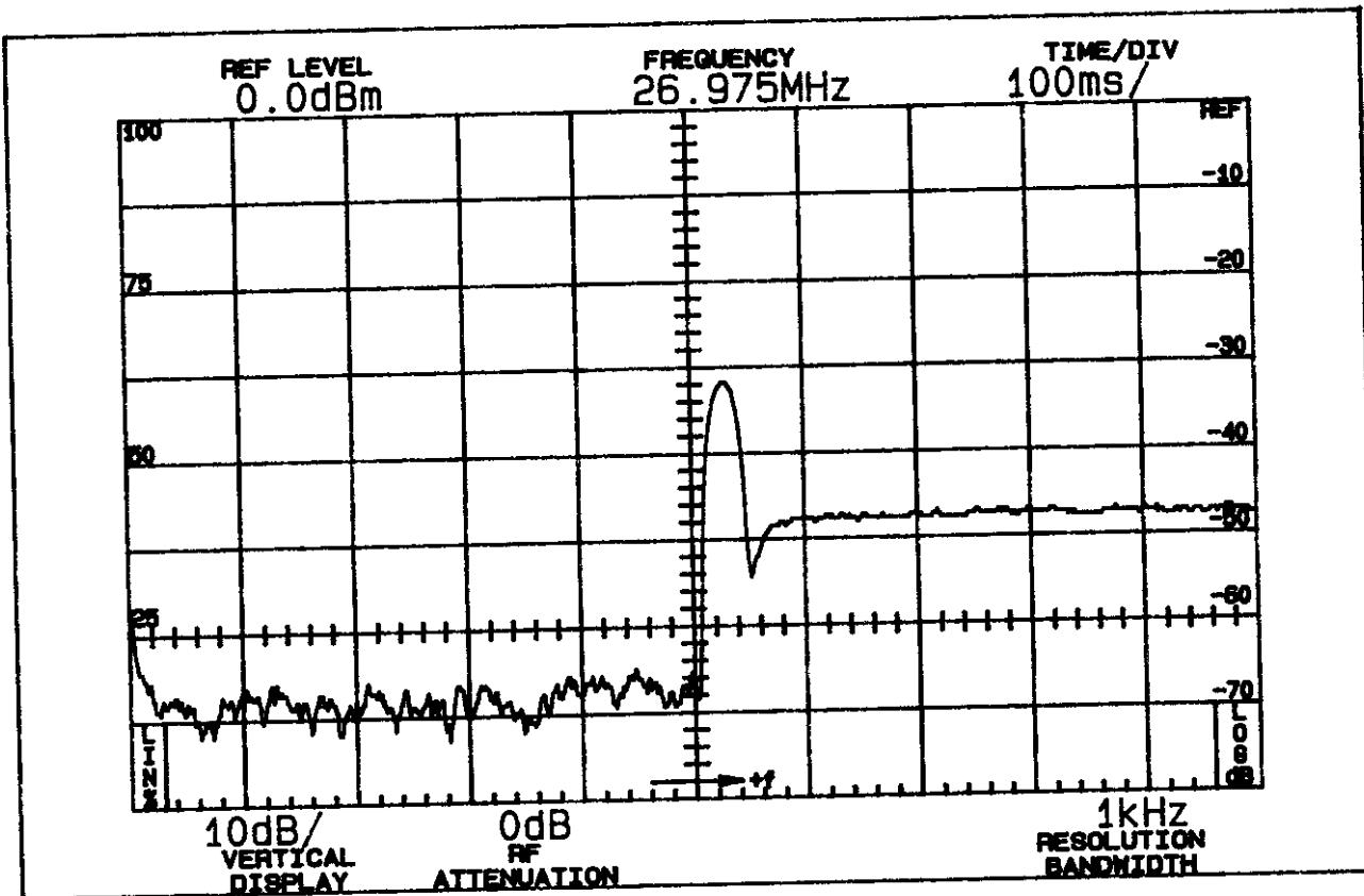
Measurement Conditions: 16 dB over 50% modulation level at 1292 Hz with 2500 Hz tone, upper fourth order sideband; horizontal scale 100 ms/div.
