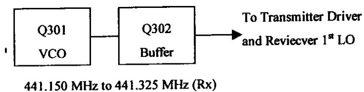
THE VCO OPERATING FREQUENCY DURING RECEIVE IS 441.150 [MHz] TO 441.325 [MHz] THE FREQUENCY IS, INJECTED THROUGH THE BUFFER AMP Q302 INTO THE FIRST LO MIXER Q109
