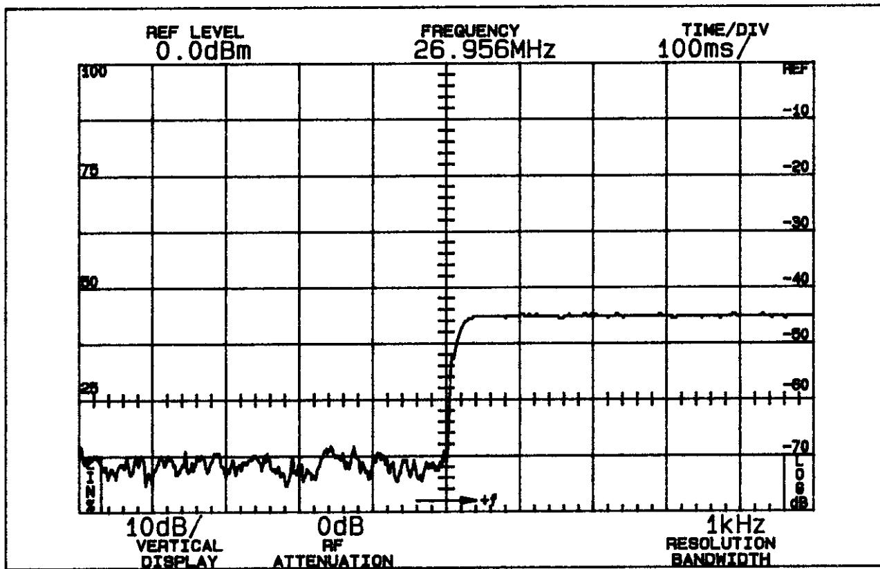
Measurement Conditions: 16 dB over 50% modulation level at 1480 Hz with 2500 Hz tone, lower fourth order sideband; horizontal scale 100 ms/div.
