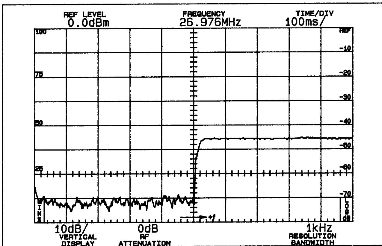
Measurement Conditions: 16 dB over 50% modulation level at 1480 Hz with 2500 Hz tone, upper fourth order sideband; horizontal scale 100 ms/div.
