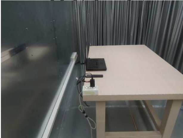
FCC 15 247 Zigbee Conduction Setup
