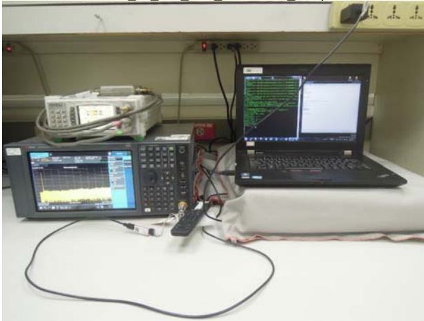
FCC 15 247 BLE Radiated Setup
