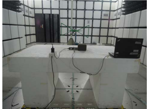
FCC 15 247 BLE Radiated Setup
