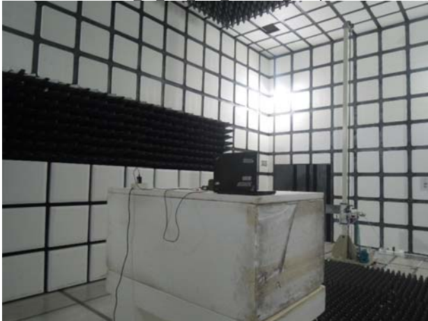
FCC 15 247 BLE Radiated Setup
