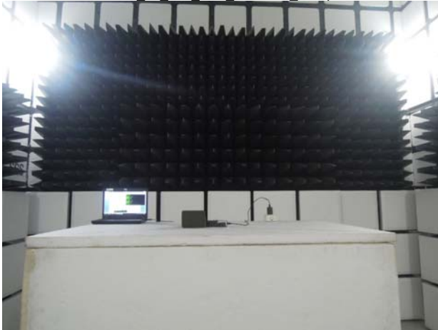
FCC 15 247 BLE Radiated Setup
