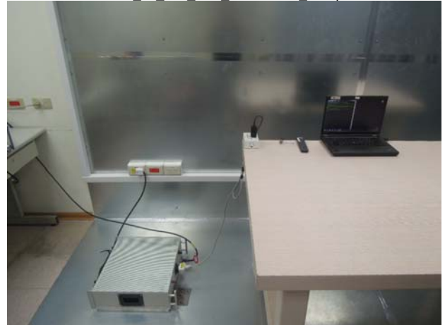
FCC 15 247 BLE Conduction Setup
