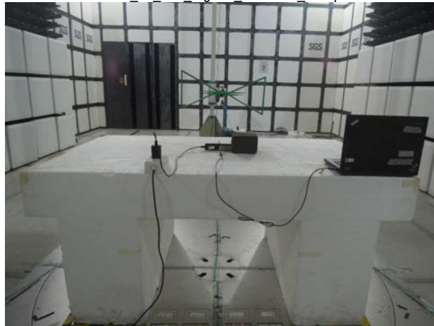
FCC 15 247 Zigbee Radiated Setup
