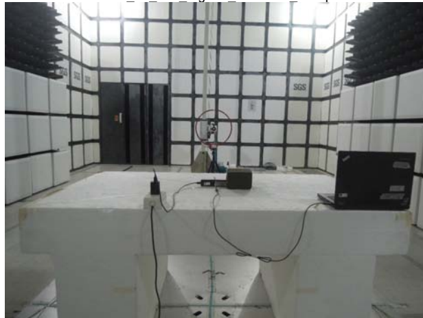
FCC 15 247 Zigbee Radiated Setup
