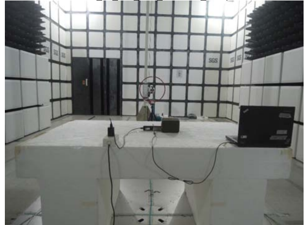
FCC 15 247 BLE Conduction Setup
