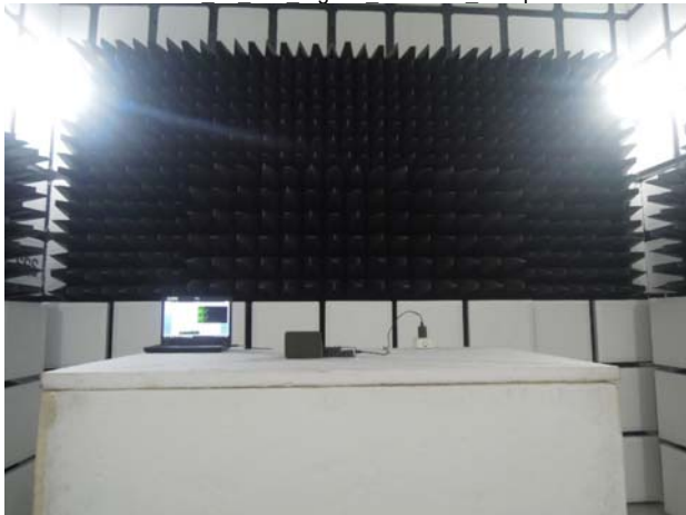
FCC 15 247 Zigbee Radiated Setup
