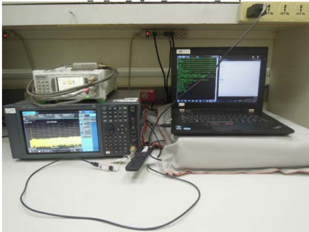
FCC 15 247 Zigbee Radiated Setup
