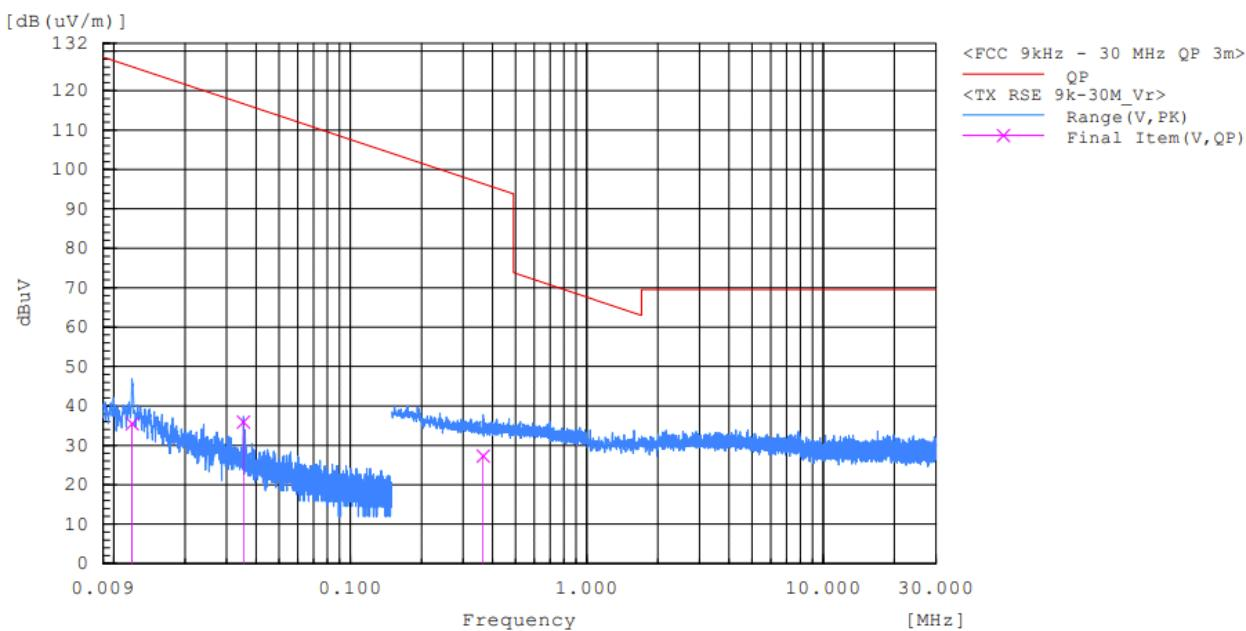
Radiated Spurious Emission 9 kHz – 30 MHz (Antenna Position 180°) : IEEE 802.15.4 (CH 11)
